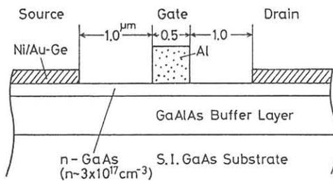
Fig.1 MESFET structure with GaAlAs buffer layer
