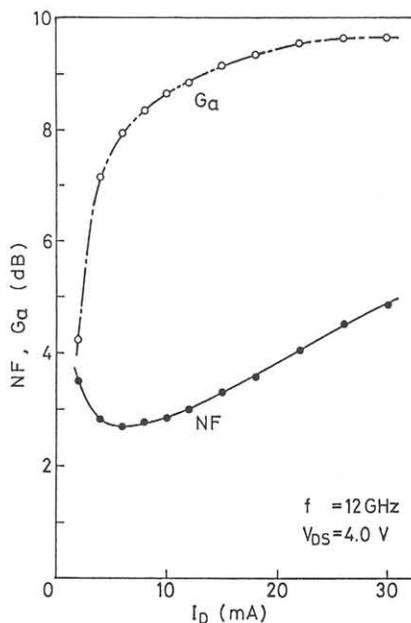
Fig.2 Drain current dependences of NF and Ga
