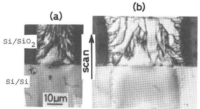
Fig. 2 Optical micrograph of a laser-irradiated sample scanned from seed to seeded area. (a) beam width: 20 μm (b) beam width: 50 μm.
