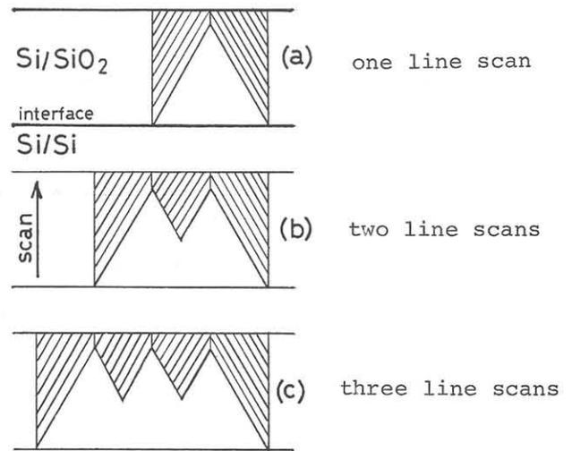
Fig. 3 Schematic illustration of recrystallization patterns of Si films on SiO<sub>2</sub> obtained by repeated scanning of Fig. 2. Beam overlapping: 50%.
