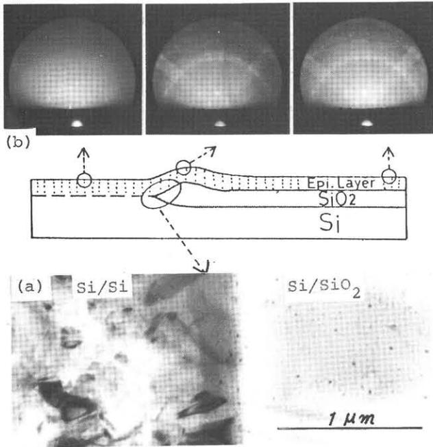
Fig. 1 Seeding effect from a small seedling area. (a) TEM micrograph showing growth differences in laser-irradiated poly-Si between Si and SiO<sub>2</sub>. (b) Schematic illustration corresponding to Fig. 1(a) and μ-RHEED observation results.
