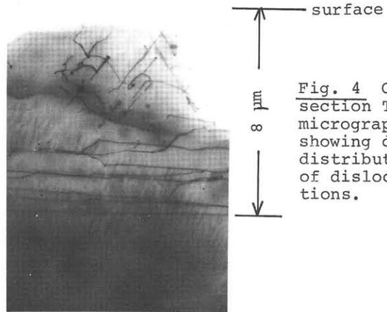
Fig. 4 Cross section TEM micrograph showing depth distribution of dislocations.
