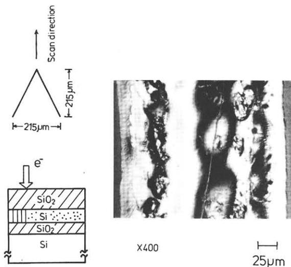
Fig.5 Recrystallized region by the V-shaped beam.
