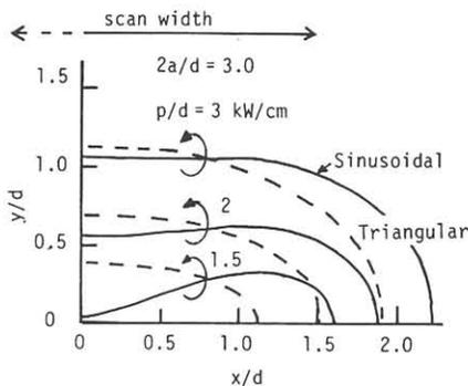
Fig.1 Contours of molten zones in Si.  $p$ : beam power,  $d$ : beam diameter,  $2a$ : scan width
