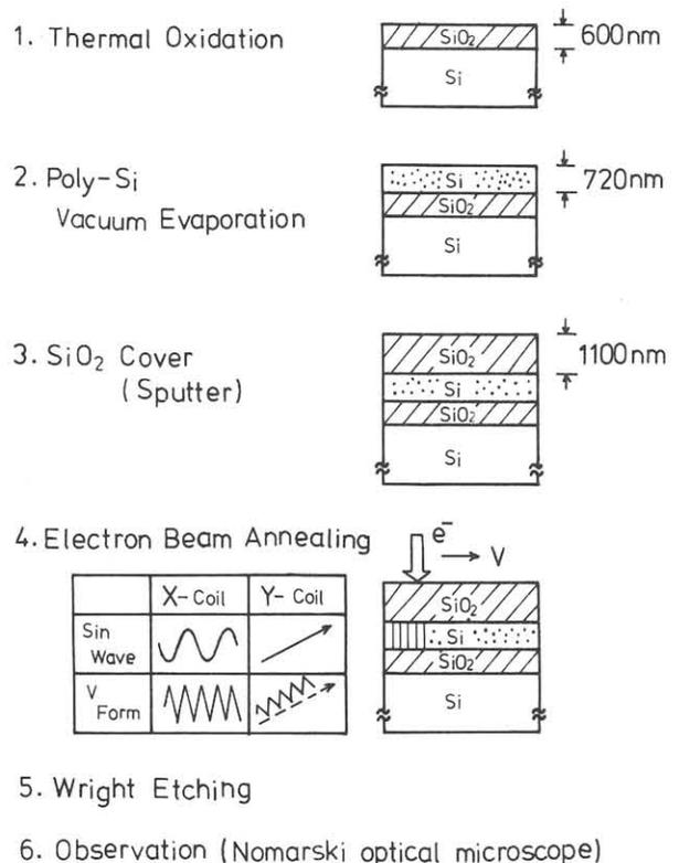
Fig.2 Experimental Procedure
