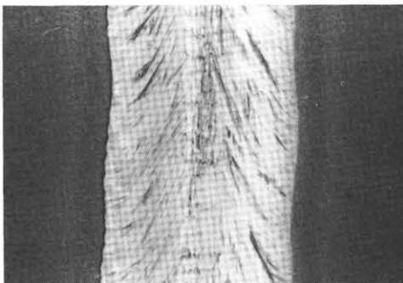
Fig.3 Nomarski optical micrograph of a Si film recrystallized by a Gaussian beam. The molten zone width is about 60  $\mu\text{m}$ .
