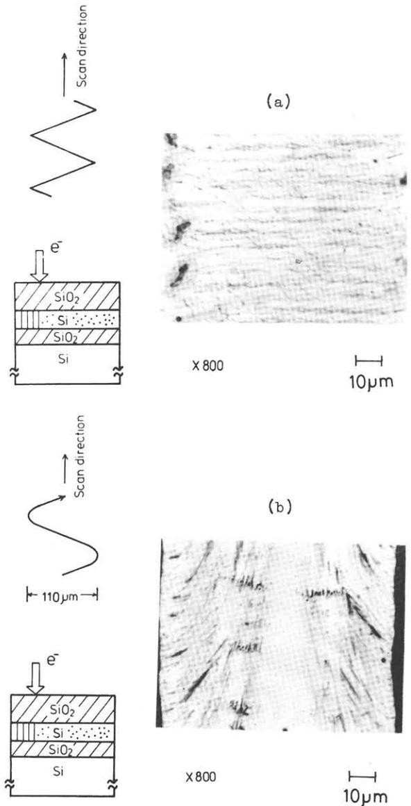
Fig.4 (a) Recrystallized region by a pseudo-line-shaped beam with triangular scanning waveform.  $V_a=30\text{kV}$ ,  $I_B=168\mu\text{A}$ ,  $d=40\mu\text{m}$ ,  $f_x=1\text{kHz}$ ,  $v_y=0.1\text{cm/s}$  and  $T_{\text{sub}}=300^\circ\text{C}$ . (b) In case of sinusoidal scanning waveform.  $V_a=30\text{kV}$ ,  $I_B=185\mu\text{A}$ ,  $d=40\mu\text{m}$ ,  $f_x=10\text{kHz}$ ,  $v_y=1\text{cm/s}$ , and  $T_{\text{sub}}=300^\circ\text{C}$ .
