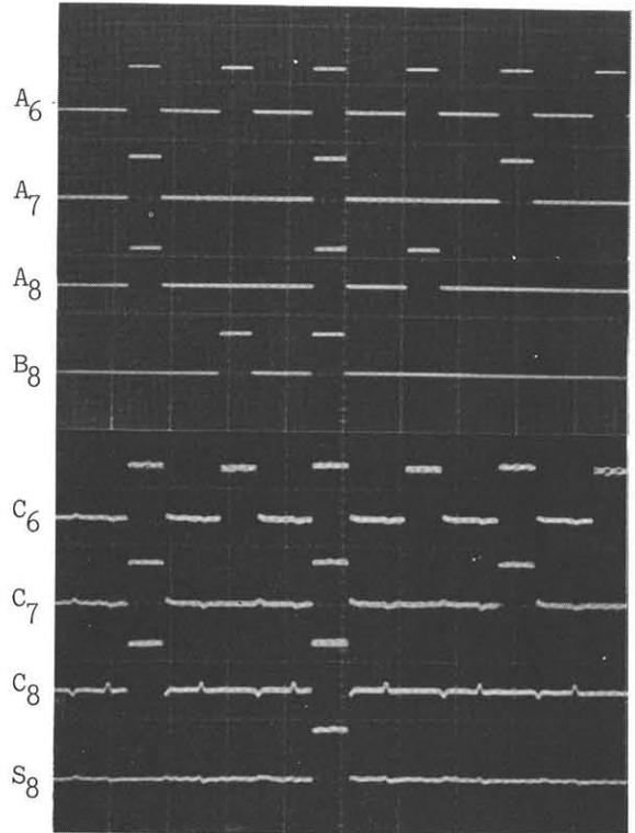
Fig.7. Examples of operations for the 8 bit RCA when ten input signals ( $A_1 \sim A_8$ ,  $B_8$  and  $C_0$ ) were applied. In this photograph four input signal ( $A_6$ ,  $A_7$ ,  $A_8$  and  $B_8$ ) and output signals ( $C_6$ ,  $C_7$ ,  $C_8$  and  $S_8$ ) are shown.
