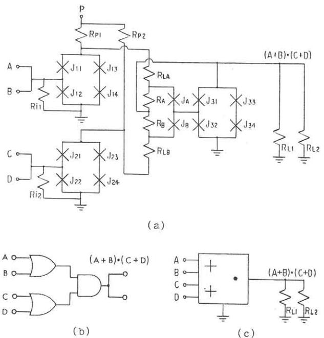
Fig.1. (a) Circuit diagram of the OR-AND cell, (b) its logic diagram and (c) symbolic notation.
