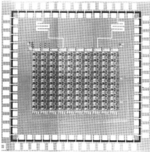
Fig.5. Photograph of a 10 X 10 cell array circuit fabricated on a 5 X 5  $\text{mm}^2$  Si chip. An 8 bit RCA circuit are wired using 56 cells in the array.
