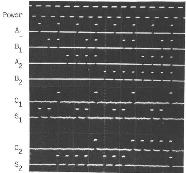
Fig.6. Full operations for the first 2 bits in the RCA obtained at a low repetition rate.
