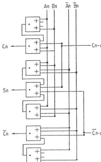
Fig.2. Circuit diagram of a 1 bit full adder used in the RCA.
