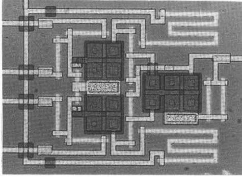
Fig.4. Microphotograph of the OR-AND unit cell fabricated using a 5  $\mu\text{m}$  lead alloy technology.
