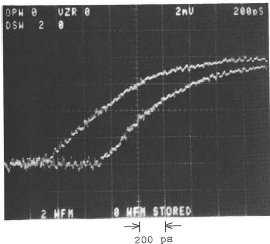
Fig.8. An experimental result of the delay measurement for the 8 bit RCA. The faster and the slower traces correspond to a bypassing signal and a propagated signal through the 8 bit RCA, respectively.
