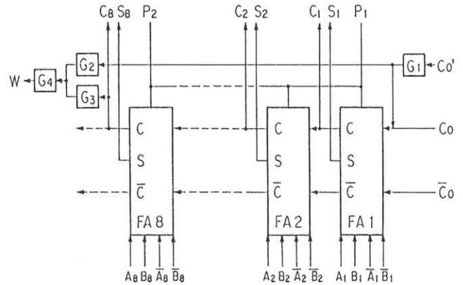
Fig.3. Circuit configuration of the 8 bit RCA. Additional four 4JL gates ( $G_1$  -  $G_4$ ) are used for measurements of carry propagation delay.
