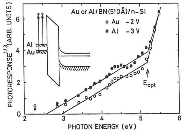
Fig. 1 Cube root of photoresponse as a function of photon energy for negatively biased MIS structures.
