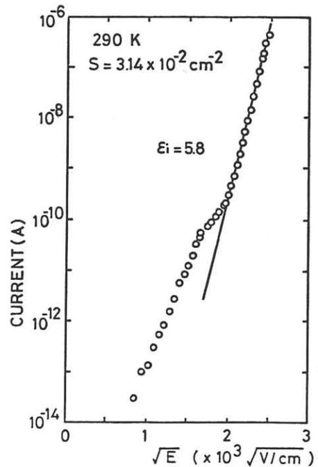
Fig. 5 Current-voltage characteristic of an Al/BN (330 Å)/Si diode.
