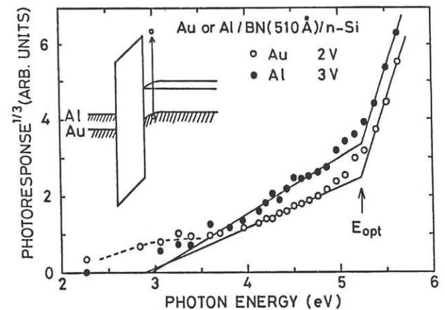
Fig. 2 Cube root of photoresponse as a function of photon energy for positively biased MIS structures.
