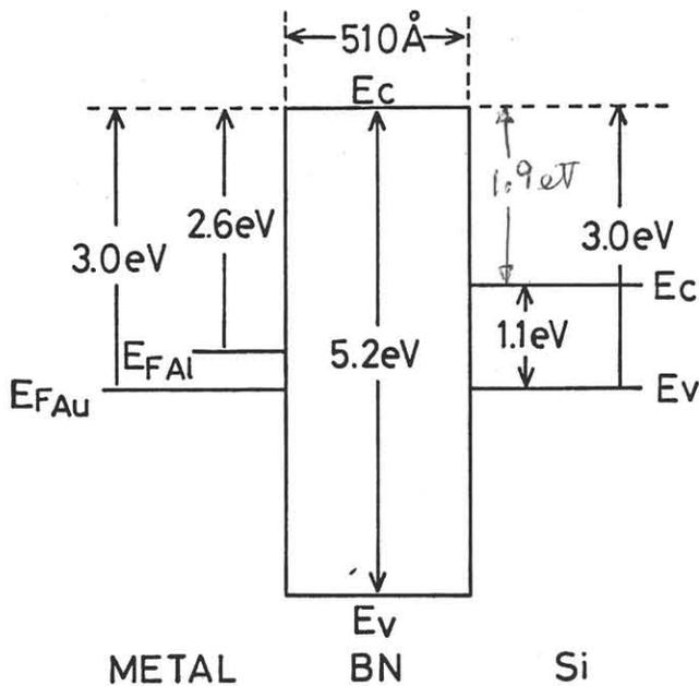
Fig. 3 Energy band diagram for a metal/BN/Si structures.
