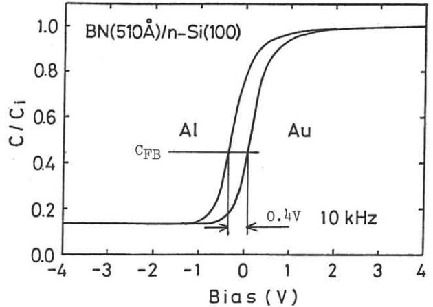
Fig. 4 Capacitance-voltage curves of MIS structures with Au and Al electrodes.
