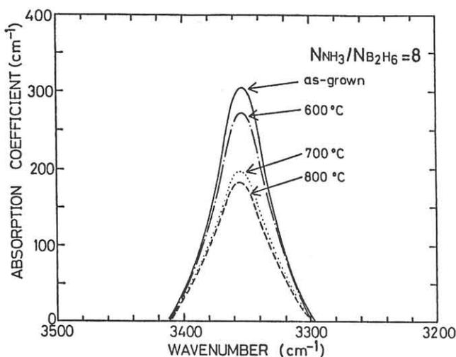
Fig. 6 Infrared absorption coefficient for the NH bonds measured after each annealing step.
