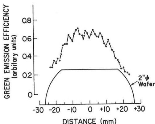
Fig. 6. Green emission efficiency distribution in GaP:N epitaxial layer using the present crystal as a substrate.
