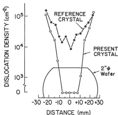
Fig. 3. Dislocation density distribution across 2 inch diameter wafers.
