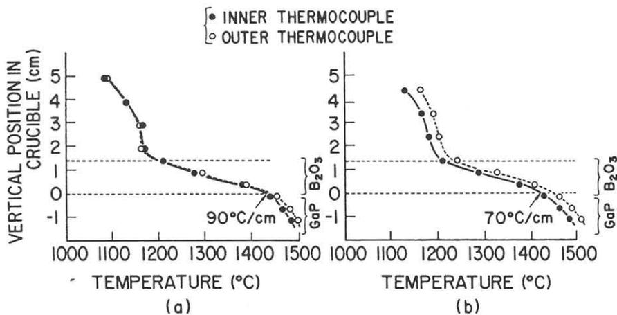
Fig. 4. Temperature distribution in crucible. (a) Present furnace. (b) Conventional furnace.
