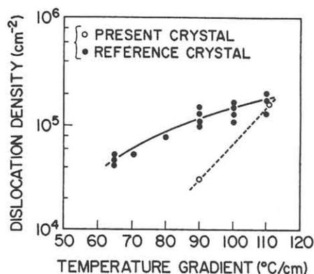
Fig. 5. Axial temperature gradient dependence of average dislocation density.
