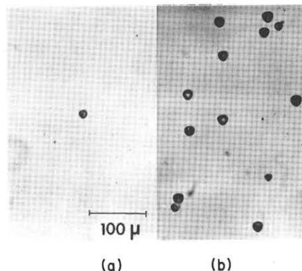
Fig. 2. Typical (111) surface etching pattern at the position of 10 mm from the center. Dislocation densities are  $10^3 \text{ cm}^{-2}$  and  $10^4 \text{ cm}^{-2}$  for (a) and (b), respectively
