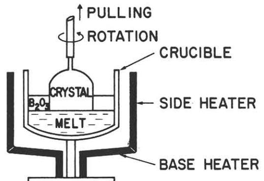
Fig.1 Schematic diagram of new heating method.
