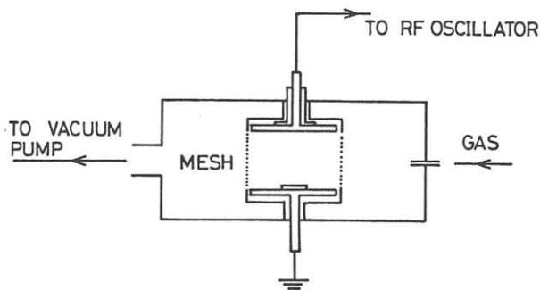
Fig.1 Experimental setup for depositing a-Si:H. RF power (9 MHz) was applied to the top electrode.
