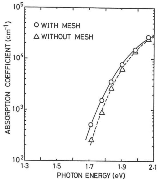
Fig. 5 Absorption coefficient as a function of photon energy for a-Si:H films obtained by various discharge apparatus.
