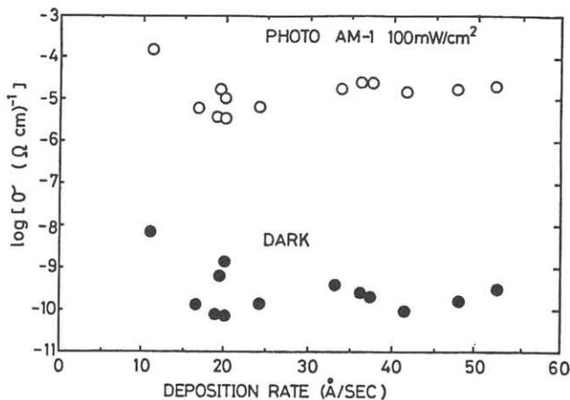
Fig. 3 Dark- and photo-conductivity of a-Si:H as a function of deposition rate.
