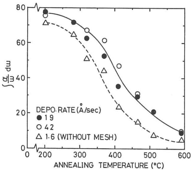
Fig. 6 Integrated intensities of the SiH stretching absorption as a function of annealing temperature.
