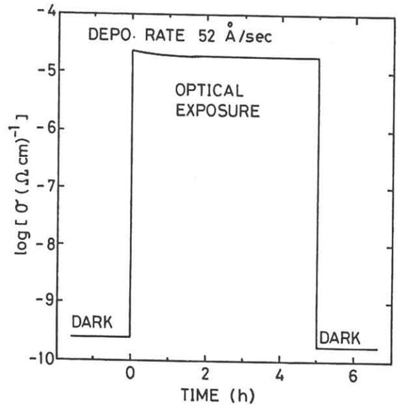
Fig. 7 Conductivity as a function of time before, during, and after exposure to 200 mW/cm<sup>2</sup> AM-1 illumination.
