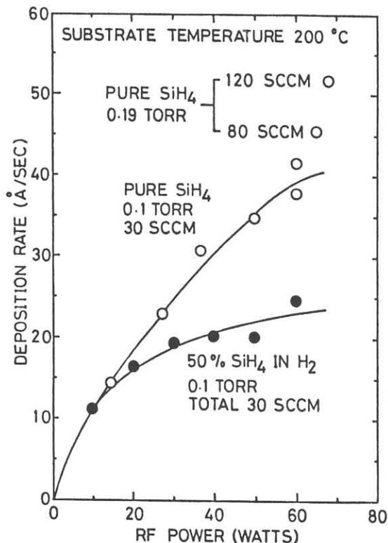
Fig. 2 Deposition rate of a-Si:H as a function of rf power.
