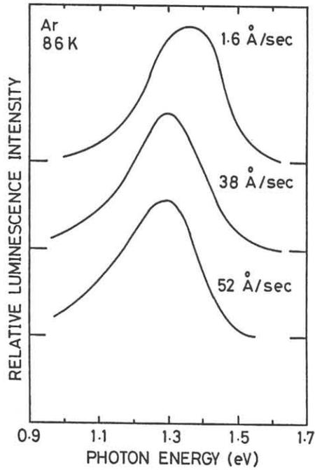
Fig. 4 Luminescence spectra for a-Si:H samples prepared at various deposition rate. Top curve refers to a specimen obtained by conventional discharge technique without mesh.
