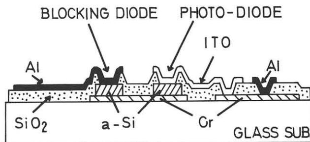
Fig. 3 Cross-section of the fabricated sensor.
