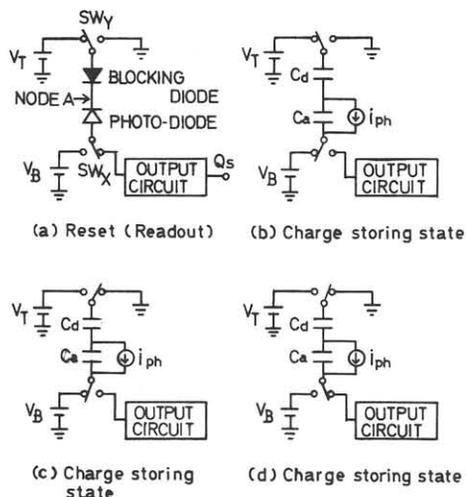
Fig. 2 Four states of the picture element.
