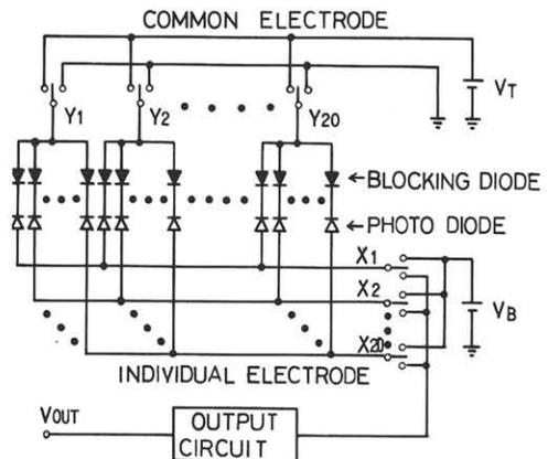
Fig. 1 Equivalent circuit configuration for the fabricated sensor.
