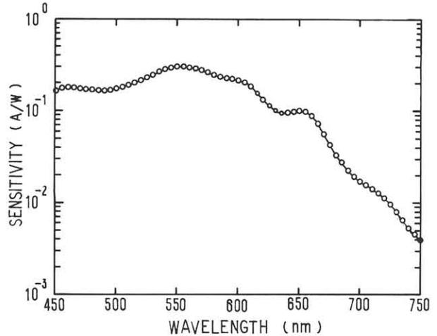
Fig. 7 Spectral sensitivity of the photo-diode.
