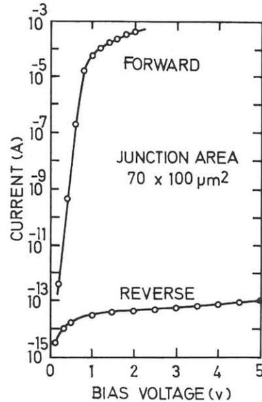
Fig. 6 I-V characteristics for the blocking diode.
