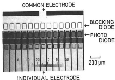
Fig. 4 Diagram of the fabricated sensor.
