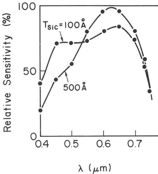
Fig.6 Relative spectral response curves for devices with different thicknesses
