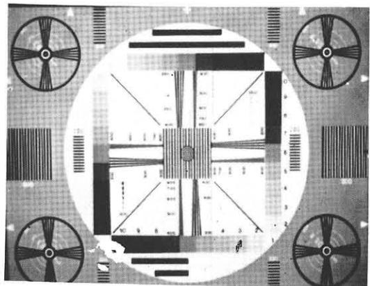
Fig.9 An image picture of a RETMA resolution chart
