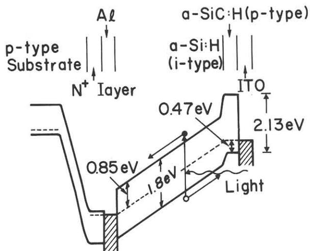
Fig.3 An energy band diagram for the photoconversion region and the storage region
