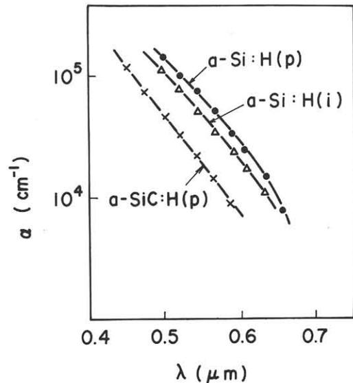
Fig.2 Absorption coefficient as a function of light wavelength
