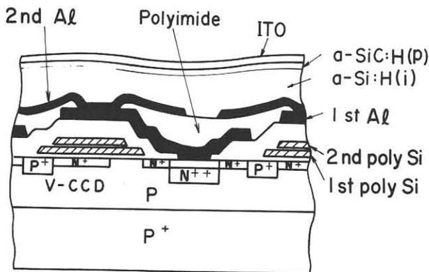
Fig.1 Cross sectional view of CCD image sensor overlaid with an a-Si:H/a-SiC:H photoconversion layer
