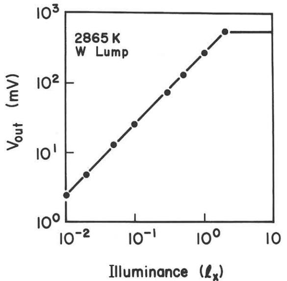
Fig.7 Device photoconversion characteristic
