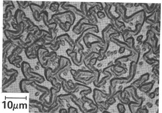
Fig.3 Etch pit pattern of GaAs grown directly on Ge(100) substrate.
