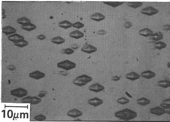
Fig.5 Etch pit pattern of single domain GaAs on Ge(100) substrate.
