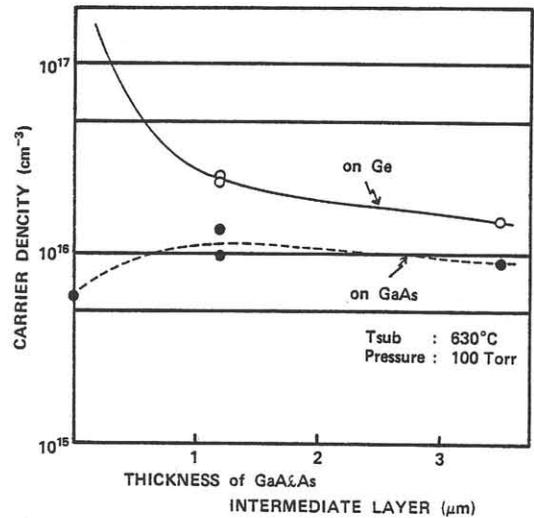
Fig.8 Carrier densities of GaAs having antiphase domain structures and GaAs on GaAs grown in the same run.
