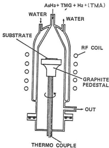
Fig.1 MO-CVD reactor used in the experiments.
