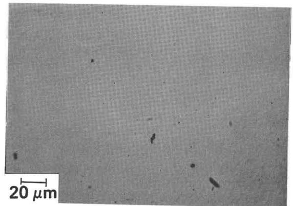
Fig.4 Surface view of single domain GaAs on Ge(100) substrate.
