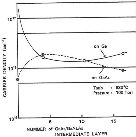
Fig.6 Carrier densities of single domain GaAs on Ge and GaAs on GaAs grown in the same run.
