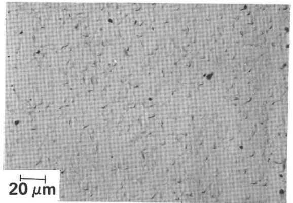
Fig.2 Surface view of GaAs grown directly on Ge(100) substrate.
