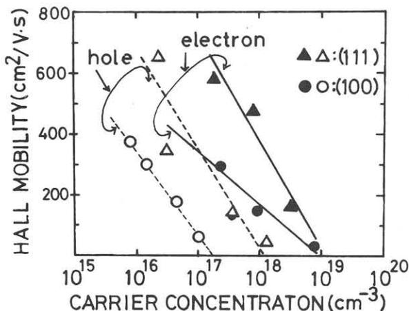
Fig.4 Hall mobility versus carrier concentration for n-type and p-type grown layer.
