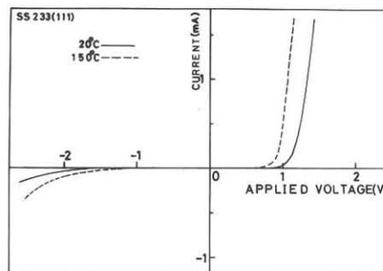
Fig.5 Current-voltage characteristics of the diode measured at 20°C and 150 °C.
