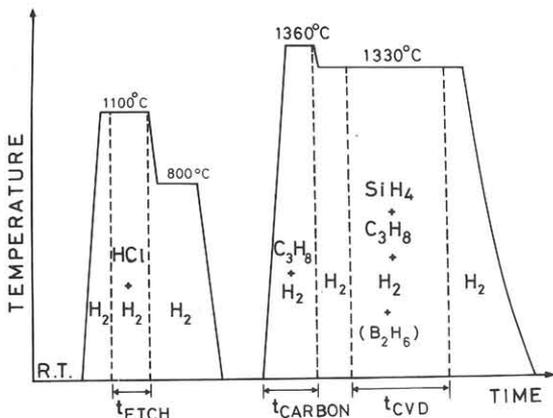
Fig.1 Temperature program of the crystal growth.
