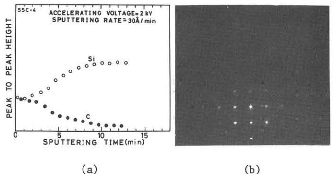
Fig.2 (a) AES depth profile of the buffer layer prepared by 2 minutes-carbonization. (b) RED pattern of the buffer layer.
