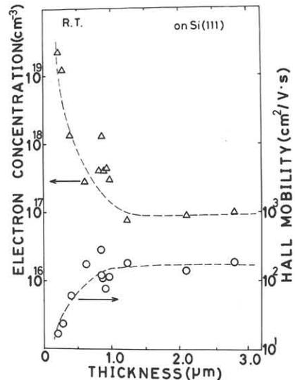
Fig.3 Carrier concentration and mobility versus thickness of the grown layer on the (111) plane: measured at room temperature.
