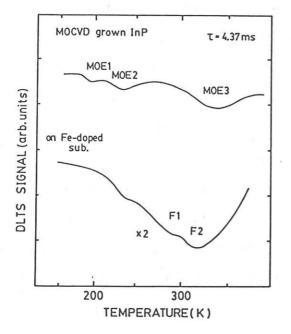
Fig. 1 Typical DLTS spectra for the InP layers grown by MOCVD on the undoped and Fe-doped substrate.
