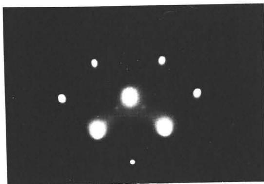
Fig. 6. RHEED patterns of  $\sim 1500 \text{ \AA}$  thick silicon film deposited on Si(100) substrate at 600 °C. The direction of the incident electron beam is  $\langle 100 \rangle$ .
