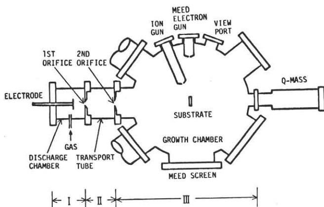
Fig. 1. Schematic diagram of RBD system.
