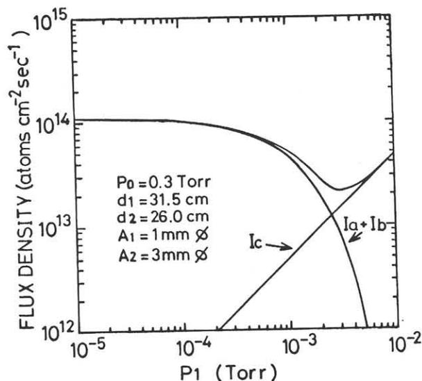
Fig. 2. Flux density as a function of the pressure in the transport tube  $P_1$ .  $d_1$  and  $d_2$  are the distance from the first orifice and from the second orifice to the substrate, respectively.  $A_1$  and  $A_2$  are the area of the first orifice and the second orifice, respectively.  $P_0$  is the pressure in the discharge chamber.
