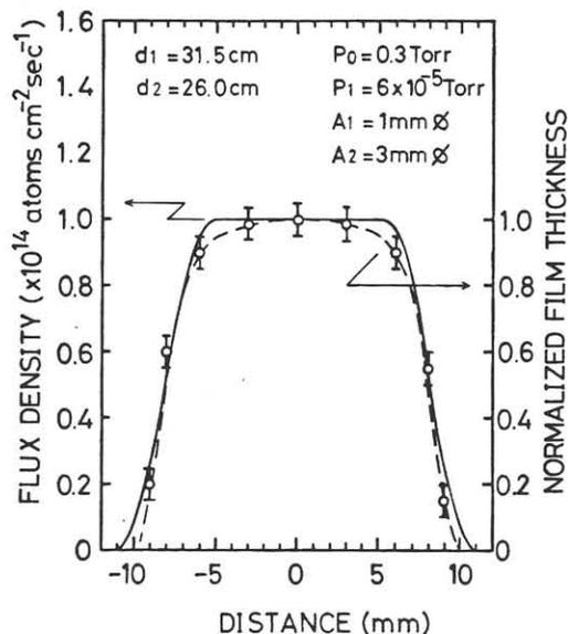
Fig. 3. Calculated beam intensity as a function of the distance from the center of the substrate (solid line) and the measured distribution of the film thickness normalized by maximum film thickness at the center is shown by dashed line.
