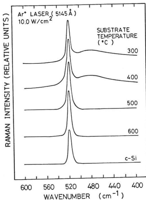
Fig. 5. Raman spectra for films grown at 300, 400, 500 and 600 °C with mirror-like morphologies and that for c-Si substrate as a reference.
