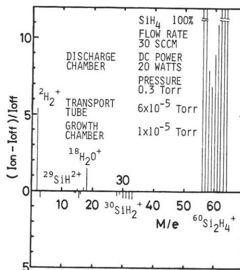
Fig. 4. The  $(I_{\text{on}} - I_{\text{off}}) / I_{\text{off}}$  ratio calculated from the mass spectra.  $I_{\text{on}}$  and  $I_{\text{off}}$  are the ion current with and without discharge, respectively.
