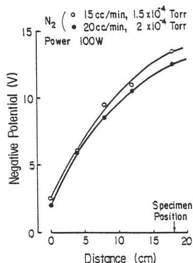
Fig. 3. Negative potential generation by divergent magnetic field method.
