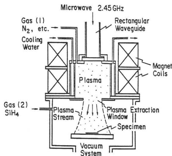
Fig. 1. ECR plasma deposition apparatus. Substrate, without heating. Gas pressure, about  $10^{-4}$  Torr.
