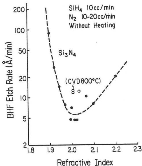
Fig. 7.  $\text{Si}_3\text{N}_4$  film etch rates with BHF solution. BHF, 50%HF:40% $\text{NH}_4\text{F}$  = 15:85,  $20^\circ\text{C}$ .
