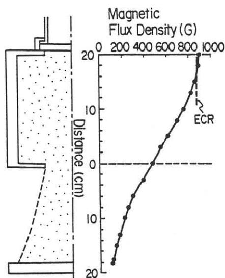
Fig. 2. Distribution of magnetic field intensity from top of plasma chamber to specimen table.
