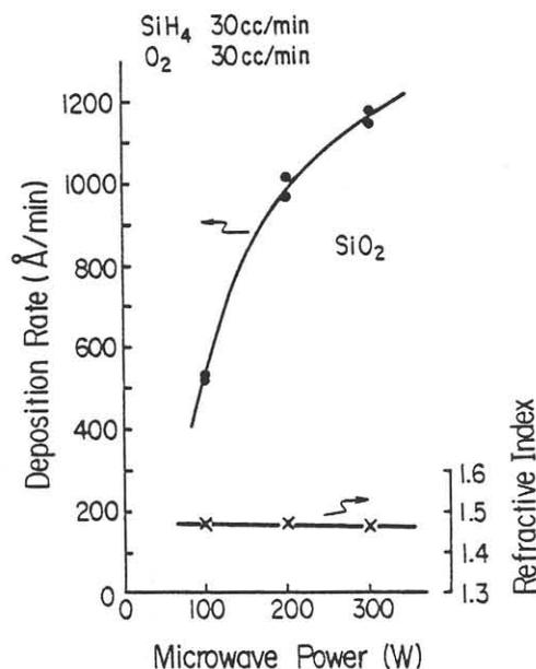
Fig. 8.  $\text{SiO}_2$  deposition characteristics.
