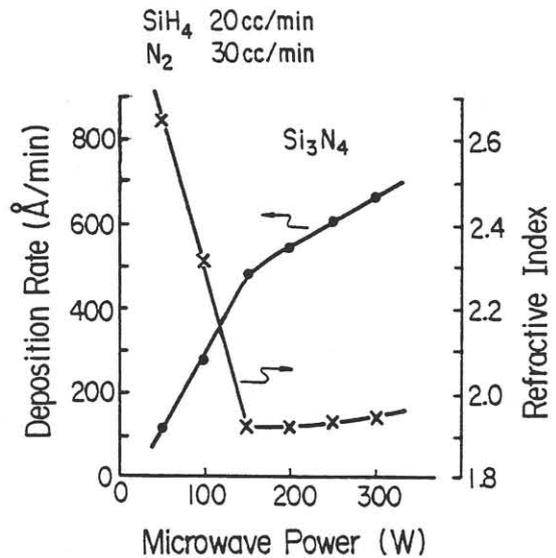
Fig. 5.  $\text{Si}_3\text{N}_4$  deposition characteristics.
