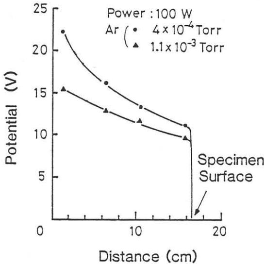
Fig. 4. Plasma potential along plasma stream.
