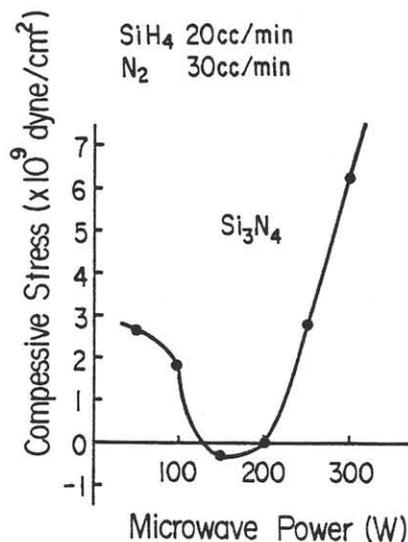
Fig. 6. Internal stress of deposited  $\text{Si}_3\text{N}_4$  films.
