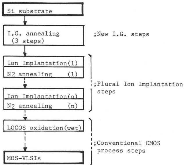
Fig. 5 CMOS process flow included I.G. steps and PIM steps.
