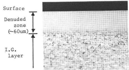
Fig. 3 Section of Si substrate after I.G. processing.
