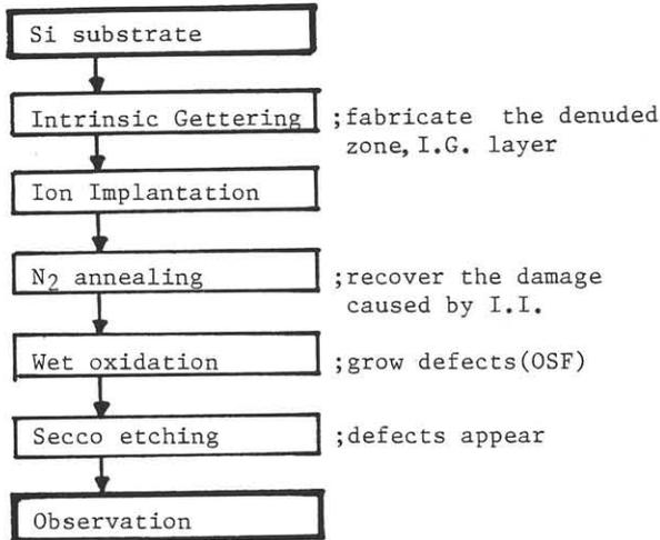
Fig. 1 Sample preparation flow.
