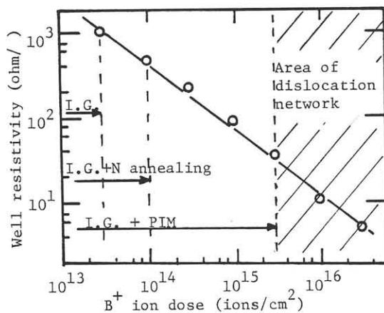
Fig. 7 Relationship between well resistivity and Boron ion dosage.
