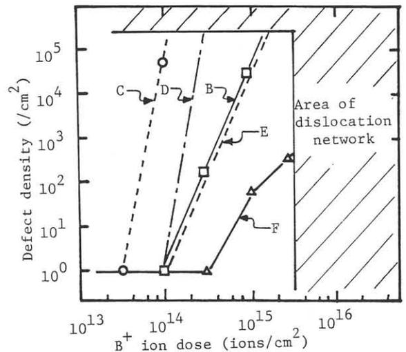
Fig. 4 Relationship between defects and Boron ion doses. Curve C:without N<sub>2</sub> annealing; curve D:N<sub>2</sub> annealing(1000 C,60min.); curve B:N<sub>2</sub> annealing(1100 C,60min.); curve E:N<sub>2</sub> annealing(1150 C,60min.) and curve F:b<sub>y</sub> Plural Ion Implantation method.
