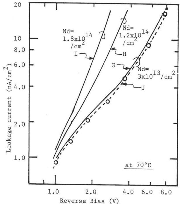
Fig. 6 Leakage current characteristics; curves G, H and I for the 3 pairs of steps, curve J for a conventional process with one pair of steps.
