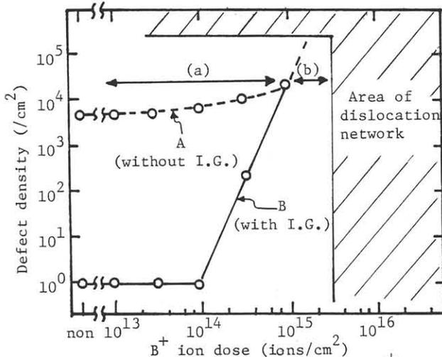
Fig. 2 Relationship between defects and B<sup>+</sup> ion dose. Line A:non I.G. ;line B:I.G.
