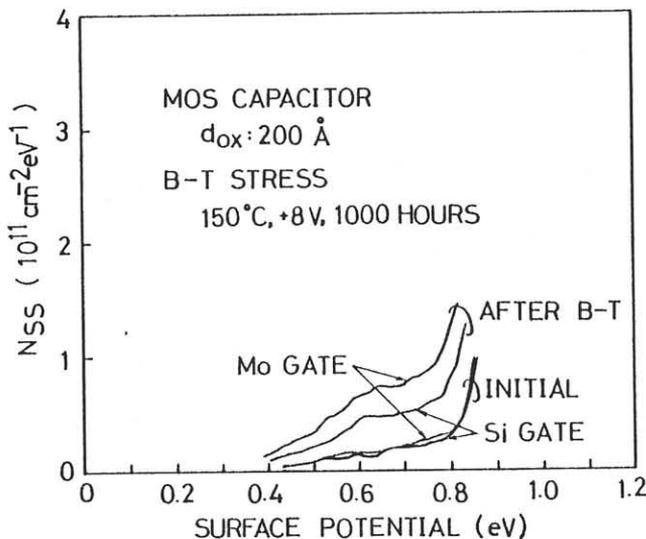
Fig.3 Surface states of Mo gate MOS capacitors before and after B-T stress aging.
