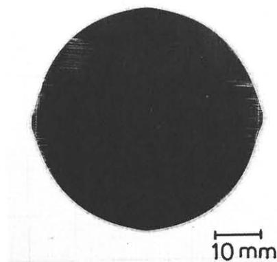
Fig. 6 Photograph of a typical wafer, cut from the 50 mm diameter crystal grown by the FEC technique with indium doping after KOH etching.
