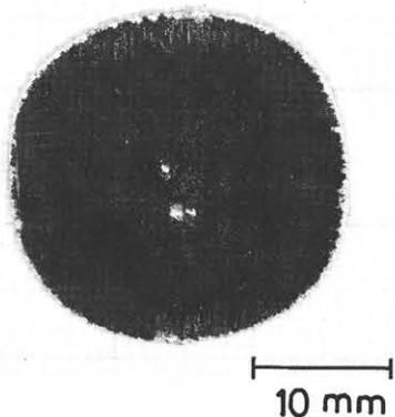
Fig. 4 Photograph of a wafer cut from the crystal grown by the conventional LEC technique with indium doping after KOH etching. White regions on the wafer correspond to dislocations.
