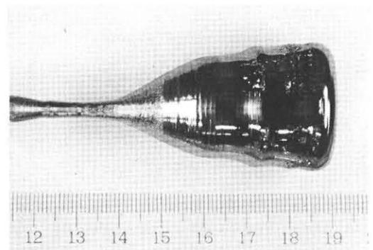
Fig. 2 Photograph of a crystal grown by the FEC technique in combination with indium doping. Crystal diameter and length are about 25 and 50 mm, respectively.
