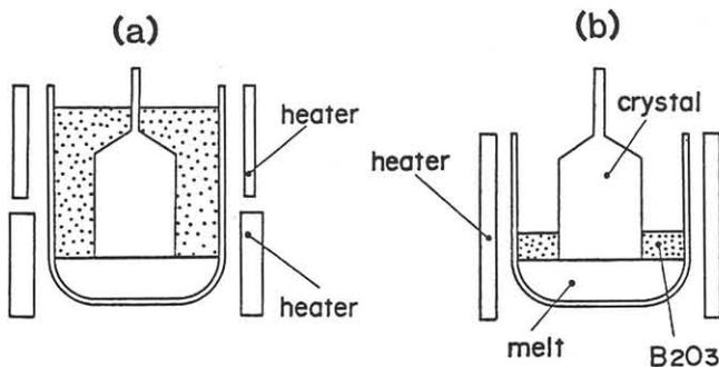
Fig. 1 Schematic drawing of the experimental setup. (a) FEC method. (b) Conventional LEC method.
