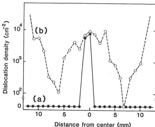
Fig. 5 Radial variations in dislocation densities measured in the  $\langle 110 \rangle$  direction across the wafer. (a) Wafer cut from the crystal grown by the FEC technique with indium doping. (b) Wafer cut from the crystal grown by the conventional LEC technique with indium doping.
