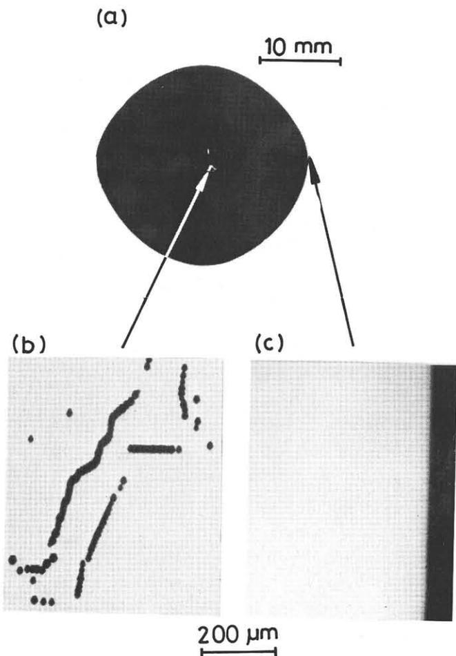
Fig. 3 (a) Photograph of a wafer cut from the crystal grown by the FEC technique with indium doping after KOH etching. White portions in the central core on the wafer correspond to dislocations from the seed crystal. (b) Enlarged photograph of the central region indicated in (a). (c) Enlarged photograph of the peripheral region indicated in (a).
