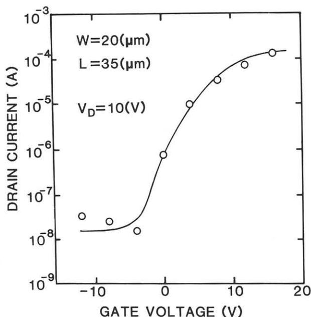
Fig. 6 Drain current vs. gate voltage characteristic at a drain voltage of  $10\text{V}$  of the same FET that shown in Fig. 5.
