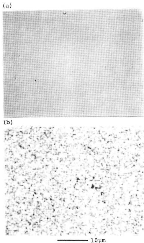
Fig. 2 Optical micrographs of surfaces of Si films grown at 800°C on CaF<sub>2</sub>/Si(111) structures with a 4nm thick predeposited Si layer (a) and without a predeposited layer (b).
