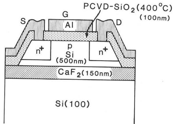
Fig. 4 Schematic cross-section of a MOSFET fabricated in the  $\text{Si}/\text{CaF}_2/\text{Si}$  structure.
