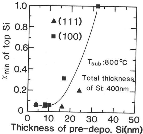
Fig. 3 Variation of the near surface  $\chi_{\min}$ 's of 400nm thick Si films grown on  $\text{CaF}_2/\text{Si}$  structures with thickness of predeposited Si layers. Si films were grown at 800°C.
