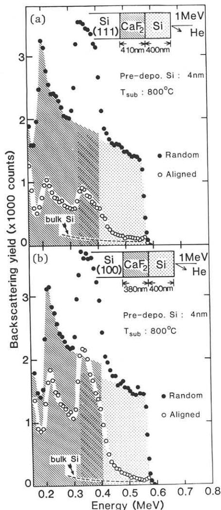
Fig. 1 Random and aligned backscattering spectra of 400nm thick Si films grown at 800°C on CaF<sub>2</sub>/Si(111) (a) and CaF<sub>2</sub>/Si(100) (b) structures predeposited with 4nm thick Si layers at room temperature. These spectra were taken with 1MeV <sup>4</sup>He<sup>+</sup> ions.
