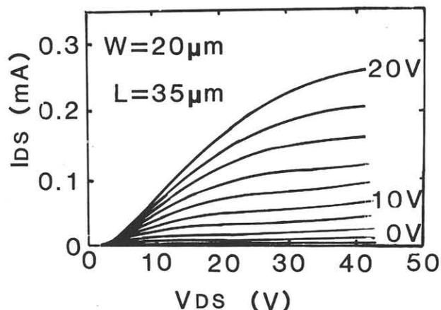
Fig. 5 Drain current vs. drain voltage characteristics of an as-prepared MOSFET with a channel length of  $35\mu\text{m}$  and a channel width of  $20\mu\text{m}$ .
