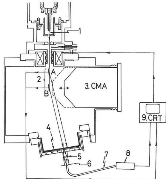
Fig.1: 1: FE tip, 2: samples, 3: cylindrical mirror analyzer, 4: fluorescent screen, 5: optical lens, 6: aperture, 7: optical fiber, 8: photo-multiplier, and 9: cathode ray tube.
