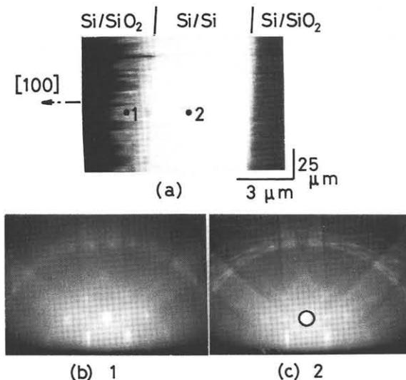
Fig.2: (a) Dark field image of an SPE sample using the 008 spot enclosed by the circle; (b) and (c) RHEED patterns from analytical points 1 and 2.
