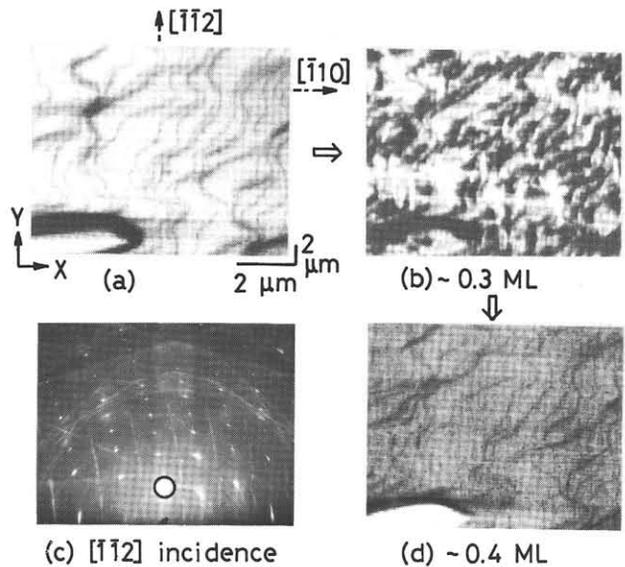
Fig.5: (a) Dark field image of a clean Si(111) surface; (b) dark field image of Au deposited surface at 800°C; (c) RHEED pattern from the dark contrast areas in (b), and (d) dark field image of the Au deposited surface.
