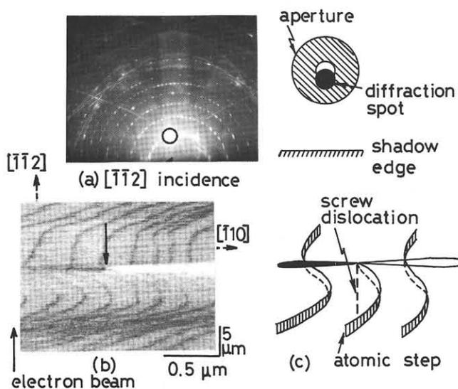
Fig.4: (a) RHEED pattern from a clean Si(111) surface; (b) dark field image of the sample using 444 spot enclosed by the circle and (c) relation between a screw dislocation and atomic steps.
