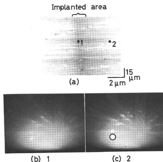
Fig.3: (a) Dark field image of an FIB sample using the spot enclosed by the circle; (b) and (c) RHEED patterns from analytical points 1 and 2.
