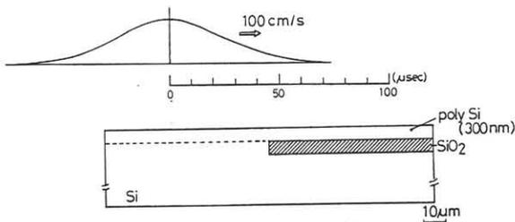
Fig.1 Simulated sample structure and beam intensity profile.
