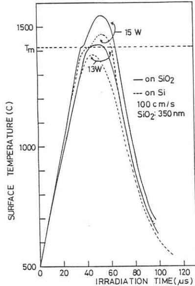
Fig.2 Laser induced surface temperature rise on poly-Si.—laser irradiation power dependence.
