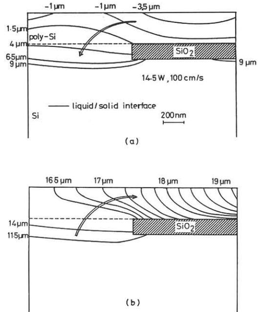
Fig.4 Movement of the liquid/solid interface in (a) melting and (b) solidification as a function of the distance from the SiO<sub>2</sub> edge to the center of the laser beam for thin (150nm) SiO<sub>2</sub> layer.
