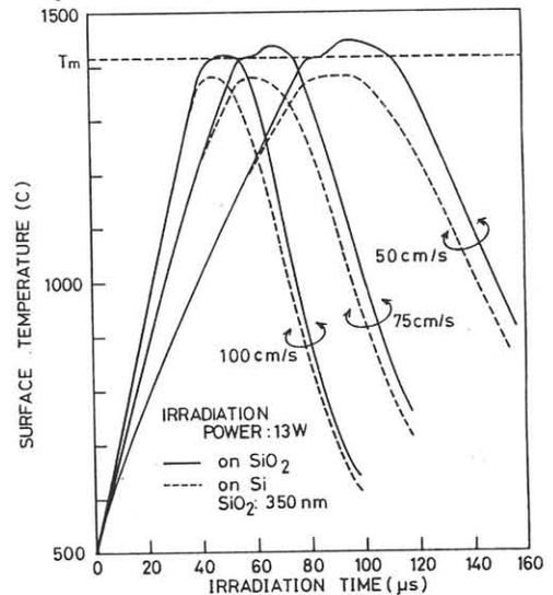
Fig.3 Laser induced surface temperature rise on poly-Si.—beam scanning speed dependence.
