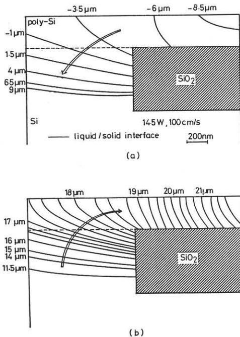
Fig.5 Movement of the liquid/solid interface in (a) melting and (b) solidification as a function of the distance from the SiO<sub>2</sub> edge to the center of the laser beam for thick (600nm) SiO<sub>2</sub> layer.
