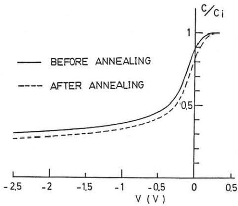
Fig. 4 MIS C-V characteristics before and after annealing process.
