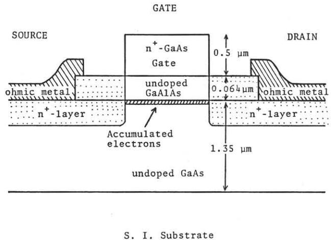
Fig.1 Schematic structure of GaAs MIS-like FET.
