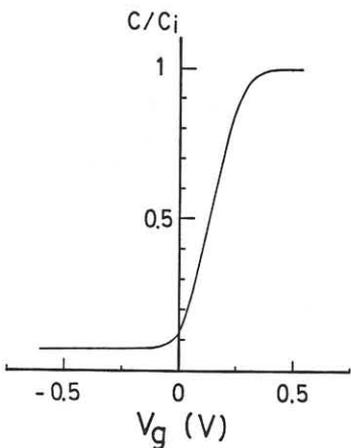
Fig. 5 MIS C-V characteristic between gate and source electrodes of MIS-like FET.
