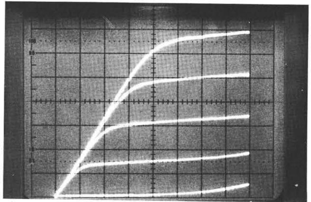
Fig. 7 FET characteristics of GaAs MIS-like FET at 77K in dark. 0.4mA/div, 0.2V/div,  $V_g = 0V \sim +0.8V$  (0.2V step).
