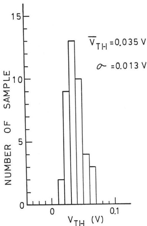
Fig.8 Distribution of threshold voltage of 41 FETs.
