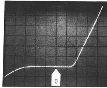
Fig. 6 Gate-source I-V curve at 77K in dark. 0.2mA/div, 0.5V/div.
