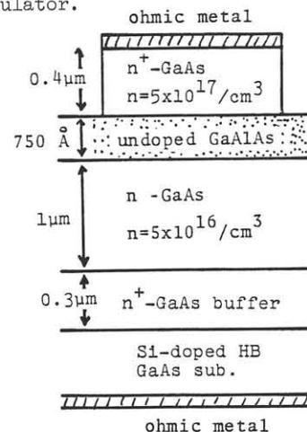
Fig.3 Schematic structure of sample for C-V measurement.
