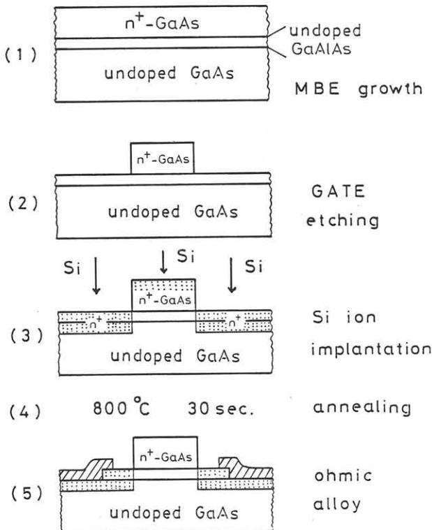
Fig.2 Fabrication process of GaAs MIS-like FET.
