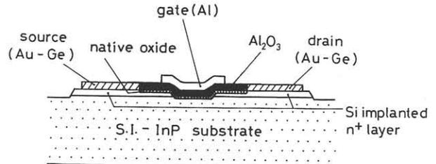
Fig. 1 Cross sectional view of the double-layer MISFET.
