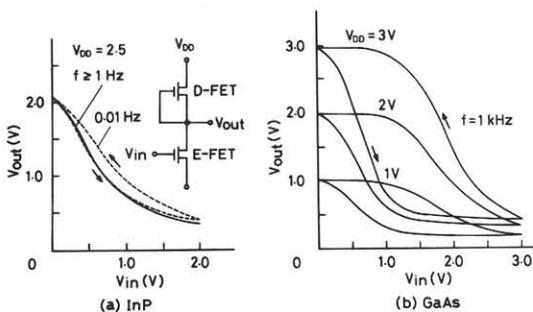
Fig. 8 Comparison of transfer characteristics between (a) InP E/D-MISFET inverter and (b) reported GaAs E/D-MOSFET inverter<sup>8)</sup>.
