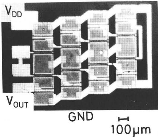
Fig. 7 Photograph of a fabricated 7-stage ring oscillator.
