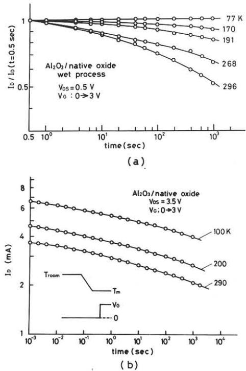
Fig. 5 Difference between temperature dependence of drift curves: data were taken by successively lowering the temperature in (a) and regaining equilibrium at room temperature before each measurement in (b).
