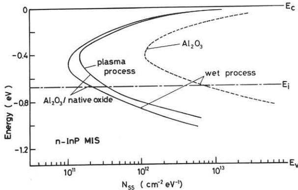
Fig. 2 Energy distribution of interface state density determined by Terman's method.
