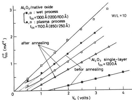
Fig. 3 Square root of drain current vs. gate voltage characteristics of MISFETs in the saturation region.
