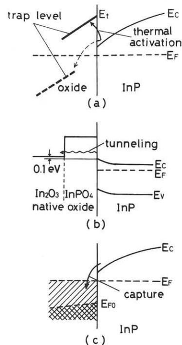
Fig. 6 Schematic band diagram illustrating the current drift: tunneling of thermally excited electrons to (a) interface traps and to (b) conduction band of  $\text{In}_2\text{O}_3$  native oxide. In (c), capture of electrons by the states under the conduction band through tunneling is illustrated.
