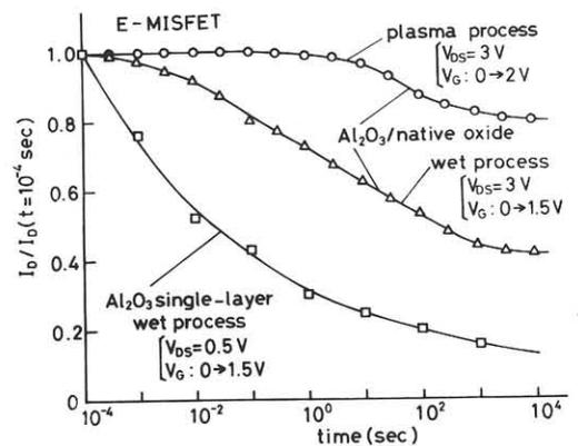
Fig. 4 Normalized drain current vs. time after application of positive gate bias.
