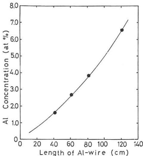
Fig.1 Al concentration of W-Al alloy versus length of Al-wire.
