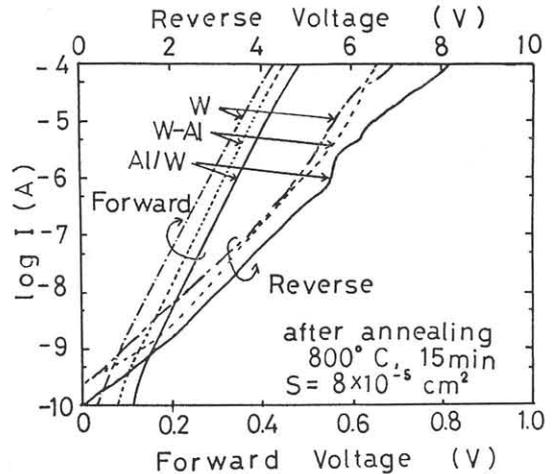
Fig.2 I-V property of W, W-Al alloy (1.7 at % Al) and Al(20 Å)/W Schottky contact to n-GaAs after  $800^\circ\text{C}$  annealing.
