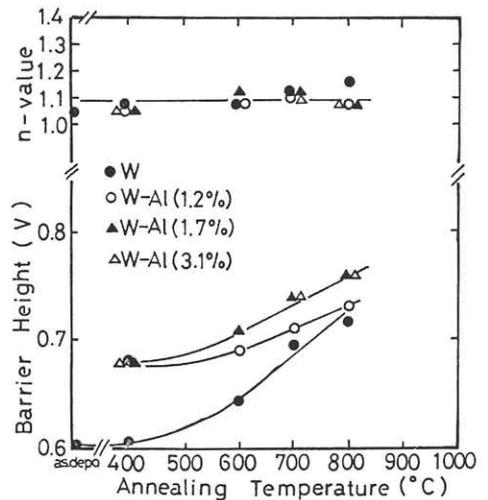
Fig.3 Annealing temperature dependence of the Schottky property using W-Al alloy film as the parameter of Al concentration.
