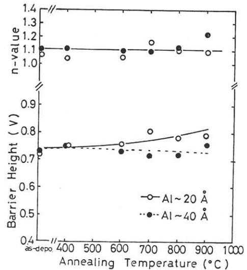
Fig.4 Annealing temperature dependence of the Schottky property using Al/W two layer metal as the parameter of Al thickness.
