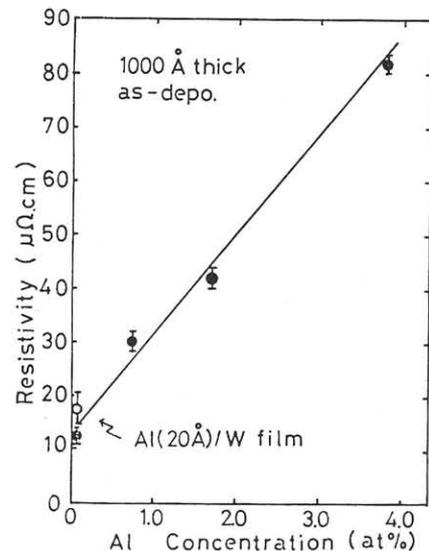
Fig.5 Resistivity of W-Al alloy film with 1000 Å thickness versus Al concentration.
