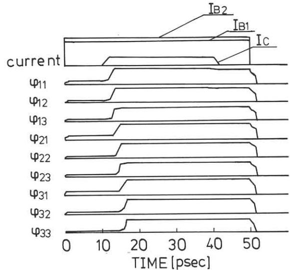
Fig.5 Simulated switching behavior of three cascaded gates, when  $I_C$  is applied to the input junction of the first gate. The parameters are the same as in Fig.3.
