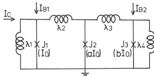
Fig.1 Proposed logic gate;  $J_1$ ,  $J_2$  and  $J_3$  are Josephson junctions,  $I_0$  is the critical current of  $J_1$ ,  $I_{B1}$  and  $I_{B2}$  are bias current, a and b are constants.
