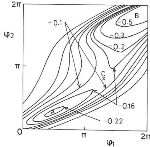
Fig.4 Contour map of potential energy for the gate in Fig.1, with the bias current. A and B are the stable points and C is the saddle point. The parameters are the same as in Fig.3, except for  $I_0=0$ .
