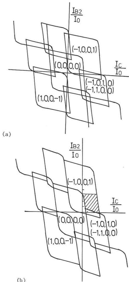
Fig.2 Calculated threshold characteristics for the gate in Fig.1, for two parameters value. The parameters are; (a)  $a=0.5$ ,  $b=2$ ,  $\lambda_1=\pi$ ,  $\lambda_2=2\pi/3$ ,  $\lambda_3=\pi/2$ ,  $\lambda_4=\pi/2$ , and  $I_{B1}=0$ . (b)  $a=1$ ,  $b=2$ ,  $\lambda_1=9\pi/10$ ,  $\lambda_2=3\pi/10$ ,  $\lambda_3=9\pi/20$ ,  $\lambda_4=9\pi/20$ , and  $I_{B1}=2.0I_0$ .
