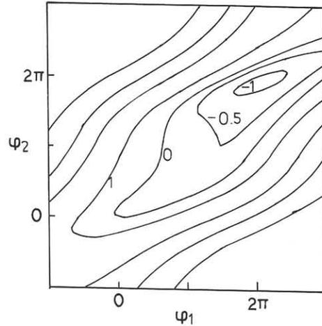
Fig.3 Contour map of potential energy for the gate in Fig.1, with the bias current and the input current. The parameters are the same as in Fig.2 (b), and  $I_{B1}=2.0I_0$ ,  $I_{B2}=2.3I_0$  and  $I_C=0.7I_0$ . The number in the figure shows the  $0$  value of potential energy for  $I_0=50 \mu A$ .
