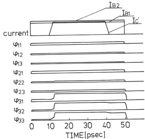
Fig.6 Simulated switching behavior of three cascaded gates, when  $I_C'$  is applied to the output junction of the third gate. The parameters are the same as in Fig.5, except for  $I_C' = 2.1I_0$ .
