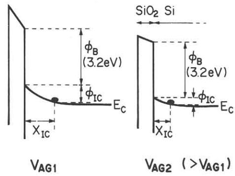
Fig.2 Effect of  $V_G$  on the potential defference  $\phi_{IC}$  and the distance  $X_{IC}$  near the drain in the saturation region.
