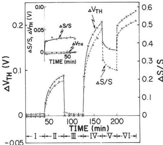
Fig.7 Changes in  $\Delta V_{TH}$  and  $\Delta S/S$  as a function of time.  $L_{eff}=0.7\mu m$ . I,III, hot-hole injection ( $V_{AG}=0.6V$ ,  $V_{AD}=5.5V$ ); II,IV,VI, hot-electron injection ( $V_{AG}=V_{AD}=5.5V$ ); V, detrapping of electrons ( $V_{AG}=-3V$ ,  $V_{AD}=0V$ ). The insert of the figure is for only hot-electron injection.
