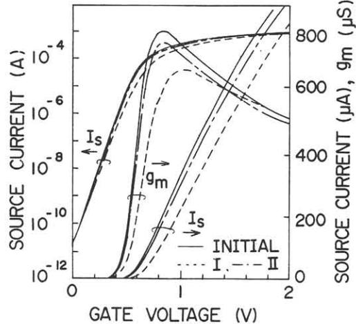
Fig. 6 Changes in source current vs. gate voltage.  $L_{eff}=0.7\mu m$ . I, after hot-electron injection for 45min ( $V_{AG}=2.2V$ ,  $V_{AD}=5.5V$ ); II, after hot-hole injection for 45min ( $V_{AG}=0.6V$ ,  $V_{AD}=5.5V$ ) following the electron injection.
