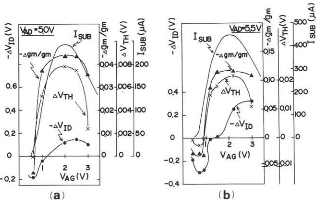
Fig.1 Dependences of stress gate voltage  $V_{AG}$  on  $\Delta V_{ID}$  and  $\Delta g_m/g_m$ .  $L_{eff}=0.7\mu\text{m}$ . (a), stress drain voltage  $V_{AD}=5.0\text{V}$ ; (b),  $V_{AD}=5.5\text{V}$ . Stress time is 90min.
