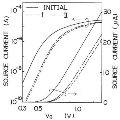
Fig. 5 Changes in source current vs. gate voltage after substrate-hot-electron injection (I) and after subsequent release (II).  $L_{eff}=1.1\mu m$ .  $V_G$ ,  $V_{SUB}$ ,  $V_D$  and  $V_S$  are 6V, -4V, OV, OV during the injection, and -3V, OV, OV, OV during the release. Each stress and subsequent release time is 60min.
