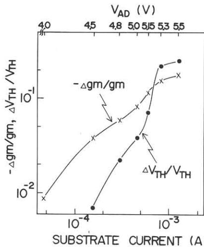
Fig. 4  $V_{TH}$  and  $g_m$  degradation ratios dependences upon the maximum substrate current for each stress drain voltage  $V_{AD}$ .  $L_{eff}=0.5\mu m$ . Stress time is 45min.
