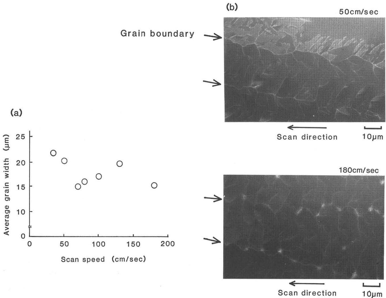
Fig.2 (a) Grain width dependence on scan speed. (b) Surface photographs after Secco etching.
