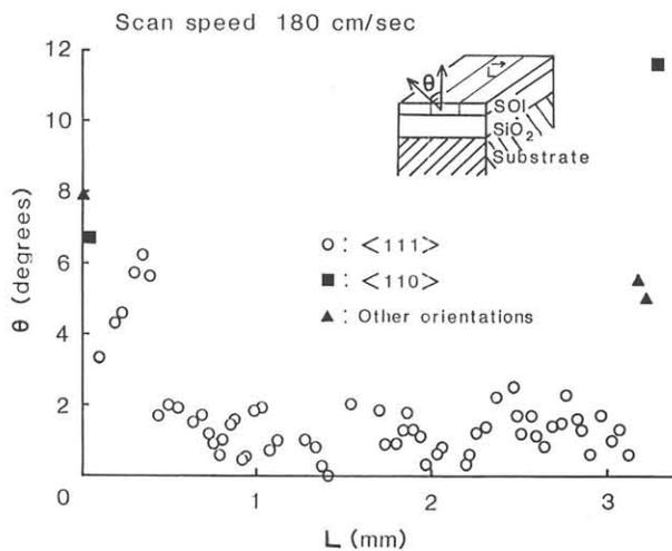
Fig.4 <111> axis deviation  $\theta$  from the surface normal direction measured along the molten width.
