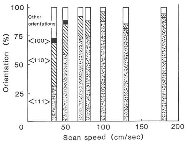
Fig.3 Crystal orientations dependence on scan speed.
