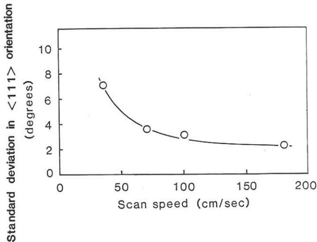
Fig.5 Standard deviation in  $\langle 111 \rangle$  orientation dependence on scan speed.
