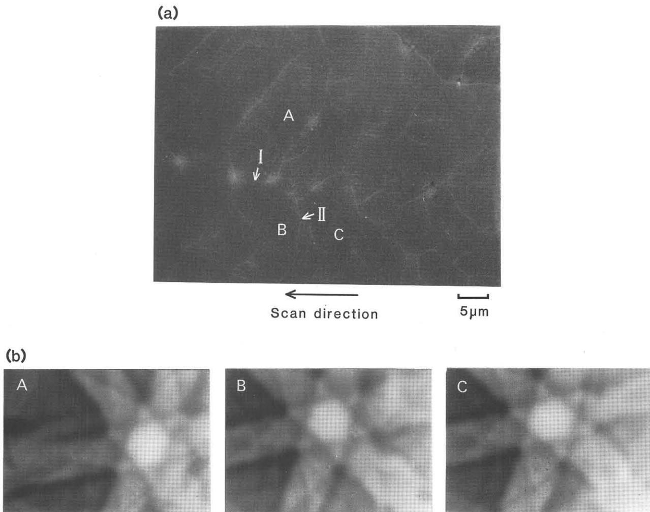
Fig.1 (a) SEM photograph of an SOI film recrystallized at 180 cm/sec. (b) ECPs corresponding to regions A, B and C.
