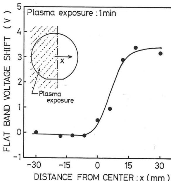
Fig. 5 Flat band voltage shift of MNOS capacitors exposed to microwave plasma.
