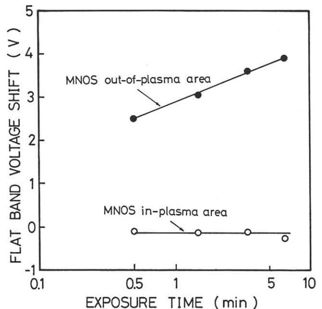
Fig. 6 Flat band voltage shift of MNOS capacitors exposed to microwave plasma as a function of exposure time.
