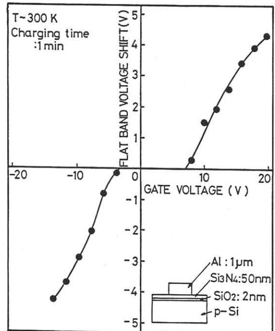
Fig. 3 Flat band voltage shift of MNOS capacitors as a function of gate voltage.
