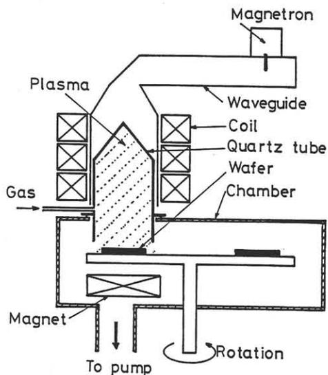
Fig. 1 Schematic diagram of microwave plasma etching equipment.
