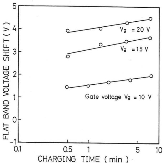
Fig. 4 Flat band voltage shift of MNOS capacitors as a function of charging time.
