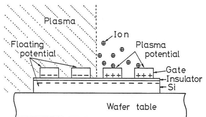
Fig. 7 Schematic representation of the charge-up mechanism for the microwave plasma etching apparatus.
