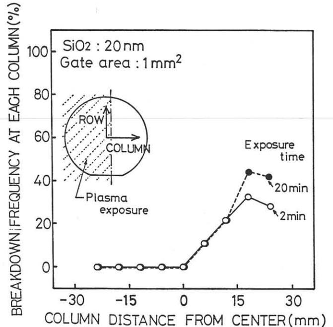
Fig. 2 Breakdown frequency of MOS capacitors fabricated on a wafer.
