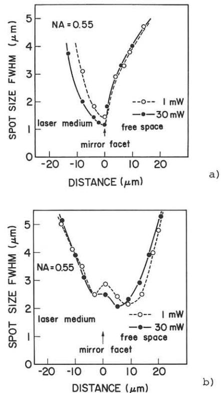
Fig.3 Position dependence of focused spot size ( $NA=0.55$  objective lens) for a) an m-ECO laser ( $1.5\mu m$  stripe), and b) an ECO laser ( $3.5\mu m$  stripe).
