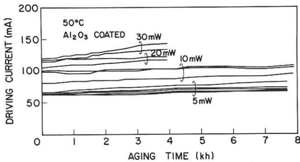
Fig.6 Aging test results for the m-ECO laser.
