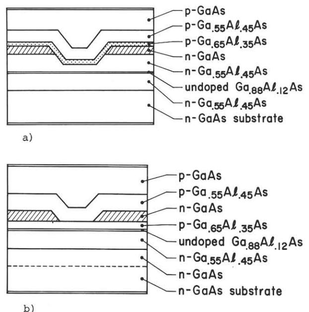
Fig.1 Schematic diagrams of a) the m-ECO and b) the ECO laser structures.
