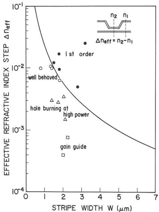
Fig.5 Transverse mode behavior of the m-ECO laser up to 30 mW as a function of the effective index step and stripe width.
