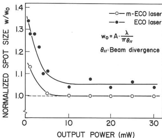
Fig.4 Output power dependence of normalized spot size for the same lasers as Fig.3.
