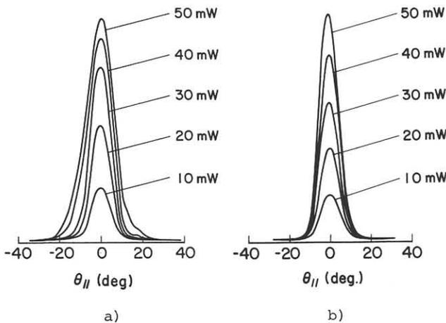
Fig.2 Far-field profiles parallel to the junction plane for a)  $1.5\mu m$  stripe m-ECO laser and b)  $3.5\mu m$  stripe ECO laser.
