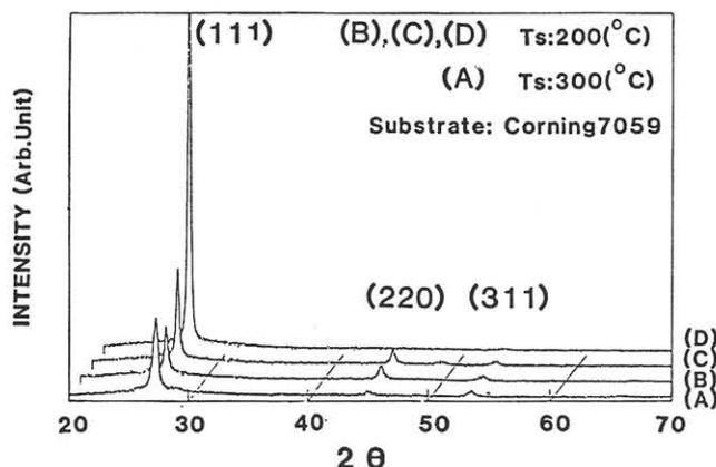
FIG. 6. X-ray diffraction curves for ZnSe films prepared at various substrate-plasma distance.
