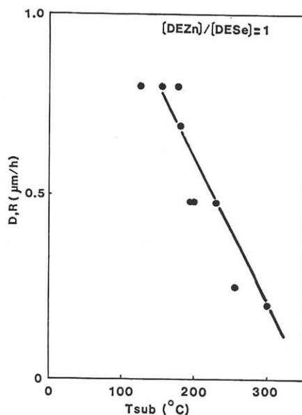
FIG. 5. The deposition rates of ZnSe films vs substrate temperature.
