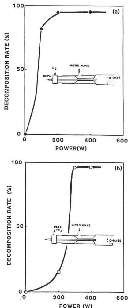
FIG. 2. The relation between the decomposition rate of source gas and microwave power for (a) DEZn and (b) DESe. The position of the gas inlet is shown in the inset.
