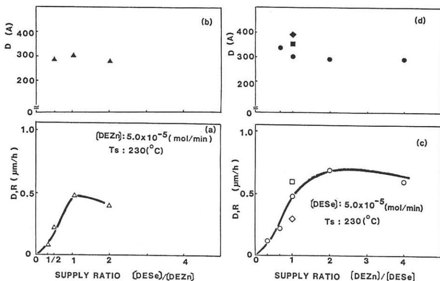
FIG. 4. (a) The deposition rates and (b) grain size of ZnSe films vs supply ratio of DESe/DEZn at a constant flow rate of DEZn. (c), (d); The same plotted as a function of supply ratio of DEZn/DESe.
