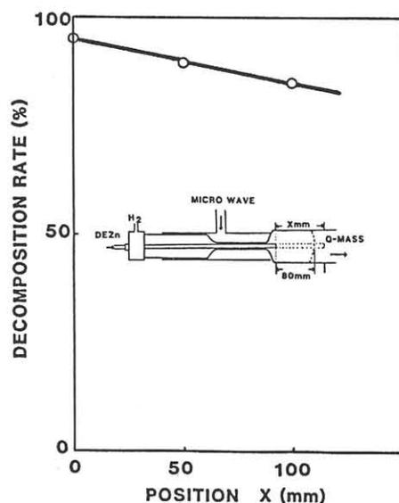
FIG. 3. The decomposition rate vs the position of the gas inlet of DEZn.
