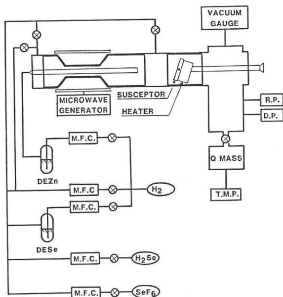
FIG. 1. Schematic diagram of apparatus used for HR-CVD of ZnSe. M.F.C.: Mass Flow Controller, R.P.: Rotary Pump, D.P.: Diffusion Pump, T.M.P.: Turbo Molecular Pump, Q-Mass: Quadrupole Mass Spectrometer.
