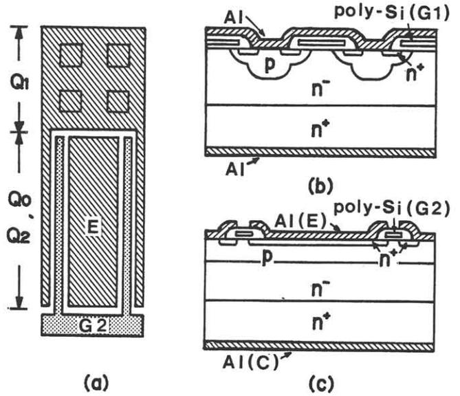
Fig.2 Structure of a unit MGT. (a) Top view.
