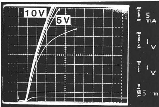
Fig.3 Static output characteristics of an MGT.
