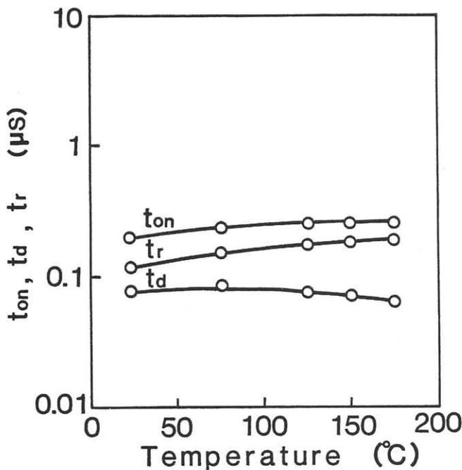
Fig. 6 Temperature dependence of turn-on times  $t_{on}$ ,  $t_d$ ,  $t_r$  of an MGT.
