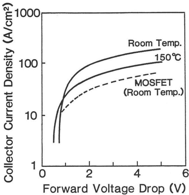
Fig. 5 Forward conduction characteristics of an MGT with a blocking voltage of 400 V. Gate voltage of the  $Q_1$  is 10 V.
