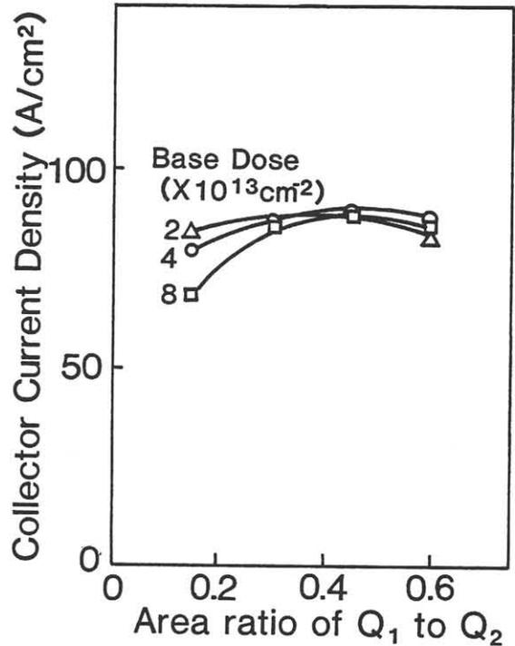
Fig.4 Conduction current density vs area ratio of  $Q_1$  to  $Q_0$ . Gate voltage of the  $Q_1$  is 10 V.
