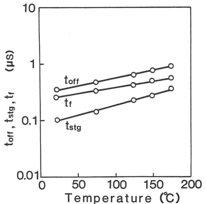
Fig. 8 Temperature dependence of turn-off times  $t_{off}$ ,  $t_{stg}$ ,  $t_f$  of an MGT.
