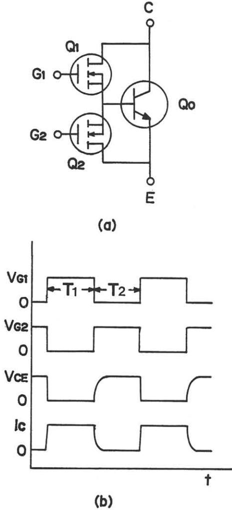
Fig.1 Equivalent circuit and operational time sequence of an MGT.
