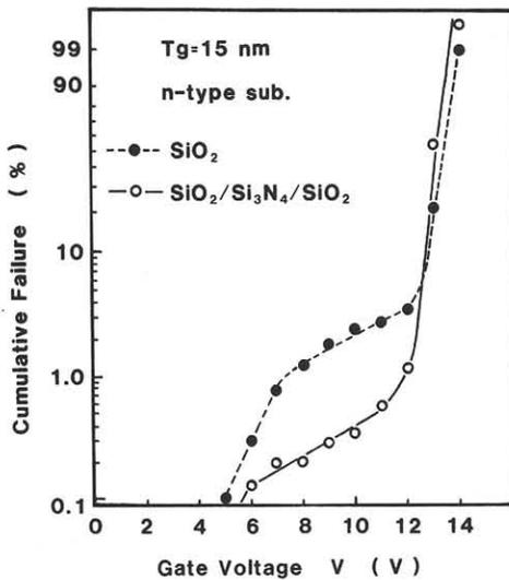
Fig.9 Time-zero dielectric breakdown characteristics of the  $\text{SiO}_2$  and  $\text{SiO}_2/\text{Si}_3\text{N}_4/\text{SiO}_2$  stacked gate.
