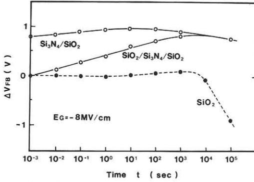
Fig.5 Relationship between  $\Delta V_{FB}$  and the aging time. The thickness of  $SiO_2$  and stacked gates are 17.7 nm and  $(1.5/1)/17.7$  nm.
