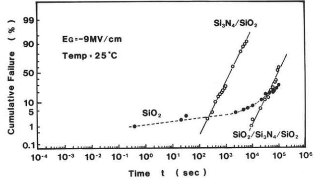
Fig.3 TDDB characteristics of the  $\text{SiO}_2$  gate (16 nm),  $\text{Si}_3\text{N}_4/\text{SiO}_2$  gate and  $\text{SiO}_2/\text{Si}_3\text{N}_4/\text{SiO}_2$  stacked gate (1.5/11/9.4 nm). (p-type sub)
