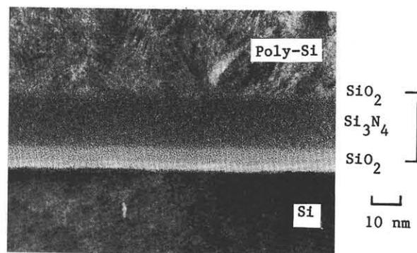
Fig.1 Cross-sectional micrograph of the SiO<sub>2</sub>/Si<sub>3</sub>N<sub>4</sub>/SiO<sub>2</sub> stacked gate.
