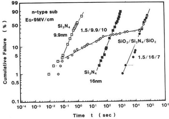
Fig.8 TDDB characteristics of the  $\text{Si}_3\text{N}_4$  gate and  $\text{SiO}_2/\text{Si}_3\text{N}_4/\text{SiO}_2$  stacked gate with the different thickness of  $\text{Si}_3\text{N}_4$  layer. (n-type sub)
