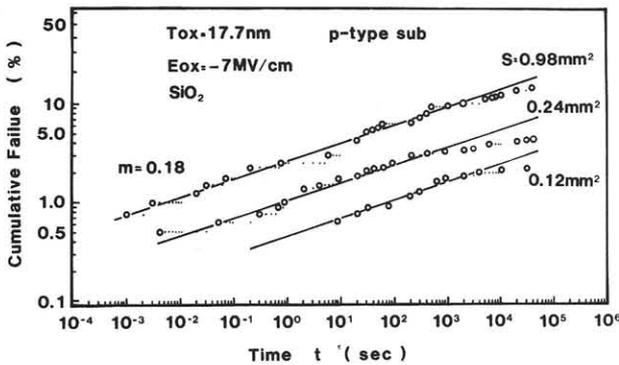
Fig.6 Weibull plot of TDDB data for the  $SiO_2$  gate (17.7 nm) under the low stress field of 7 MV/cm. The gate area  $S_g$  is a parameter.
