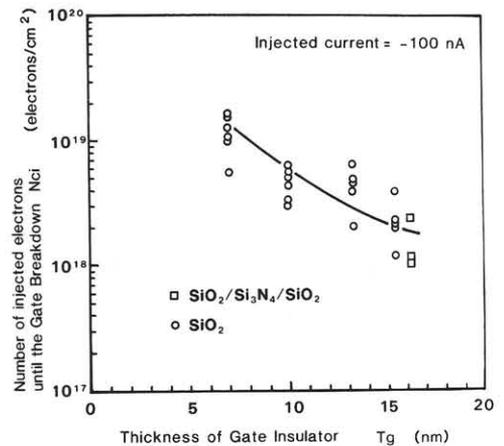
Fig.4 Gate insulator thickness dependence of the critical number of injected electrons which cause the intrinsic breakdown.
