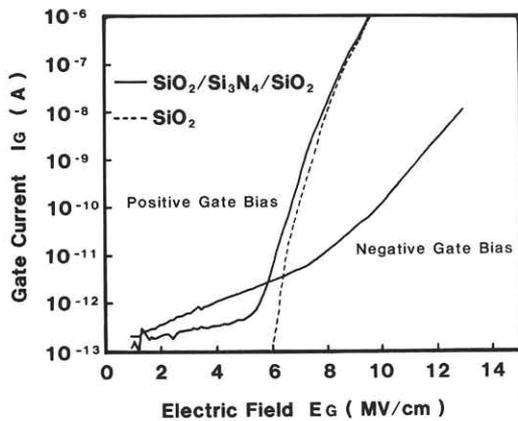
Fig.2 Gate current and Electric field characteristics. The current under positive gate bias follows F-N mechanism and that under negative bias follows P-F mechanism.
