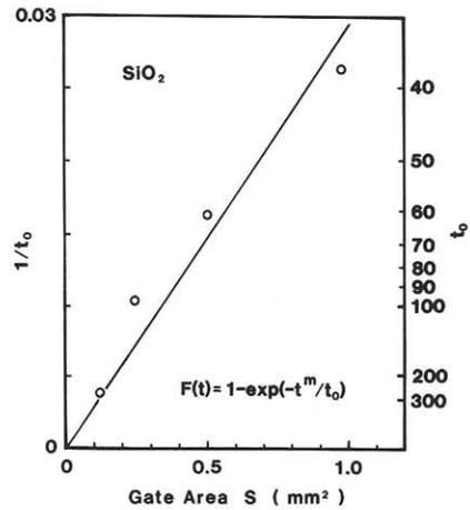
Fig.7 Relationship between Weibull parameter  $t_0$  and the gate area  $S_g$  which is calculated from the data in Fig.6.
