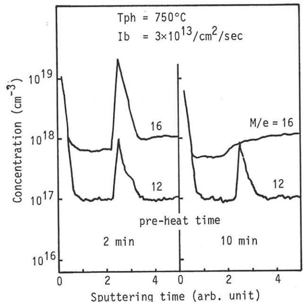
Fig. 2 Depth profiles of oxygen and carbon measured by SIMS.
