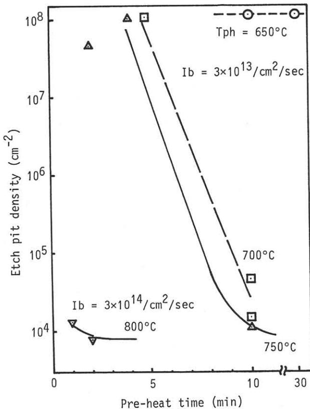
Fig. 1 Dependence of EPD on the pre-heat time at various pre-heat temperatures (Tph).  $I_b$  is a Si beam intensity.
