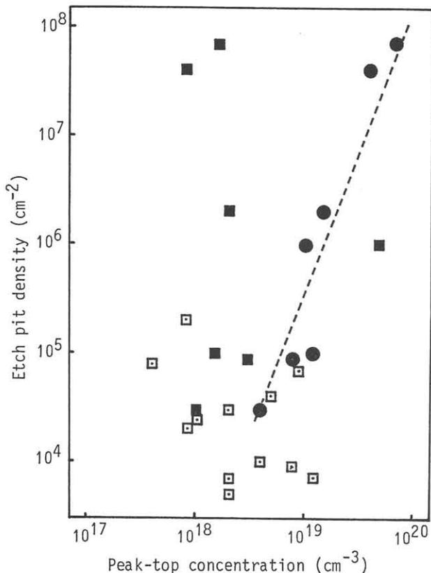
Fig. 3 Relation between EPD and peak top concentration of the interfacial oxygen (●) and carbon (□ ■).
