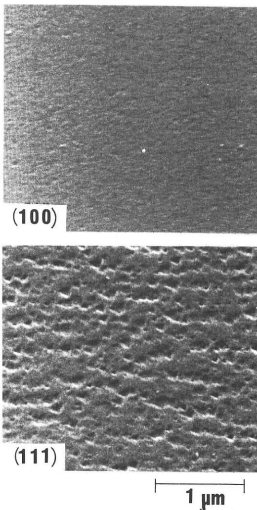
Fig. 4 SEM photographs of Sirtl etched surfaces of MBE films on (100) and (111) oriented substrates.
