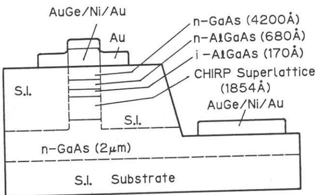
Fig. 2 Cross-sectional view of the CHIRP diode
