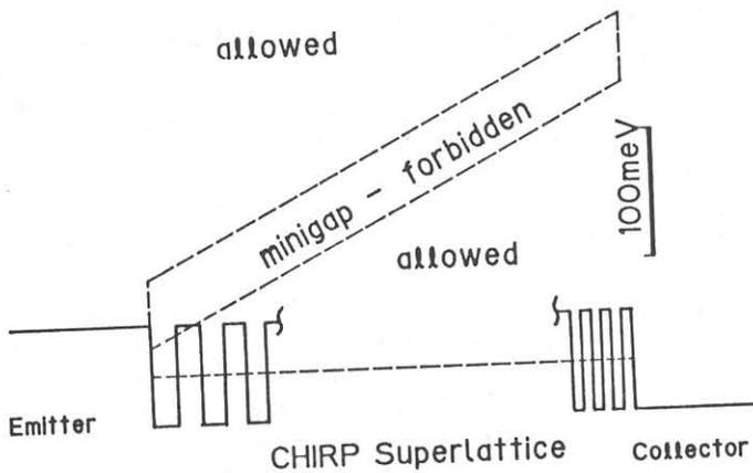
Fig. 1 Band (solid line) and miniband (broken line) structure of the CHIRP diode
