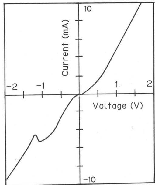
Fig. 3 I-V characteristics of the CHIRP diode
