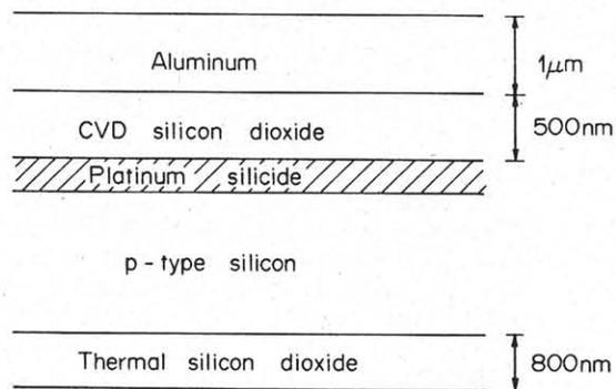
Fig.1. Optimized structure of the Schottky-barrier IR detector
