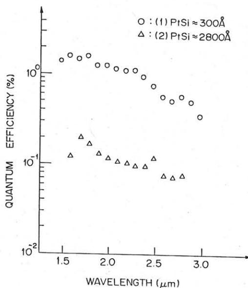
Fig.3. Quantum efficiency comparison between thin film SBD and thick film SBD
