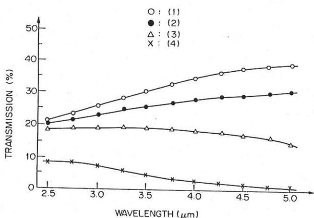
Fig.2. IR transmission with respect to the conditions of silicon-air interface (without the optical filter and PtSi film)
