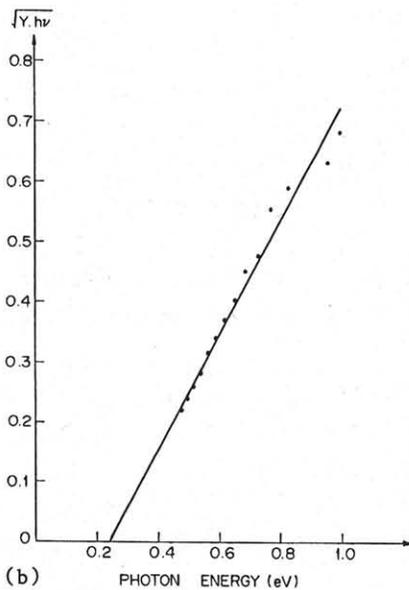
Fig.4. Modified Fowler plot for the thin film SBD's
