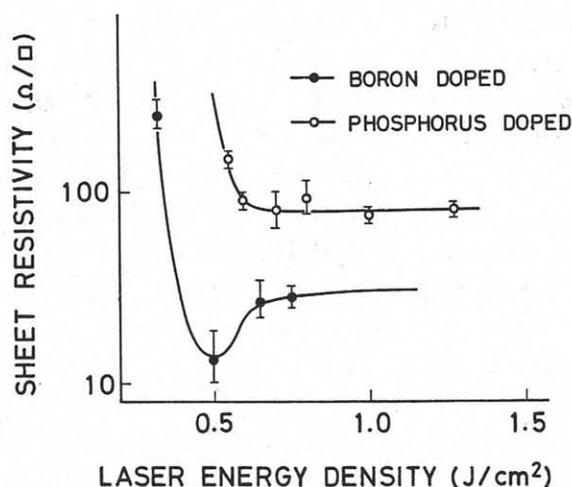
Fig. 2 Sheet resistivity of p<sup>+</sup>(solid circles) and n<sup>+</sup>(open circles) layer produced by irradiating boron/Si and phosphorus/Si surface, respectively, with 10 pulses of XeCl excimer laser beam.
