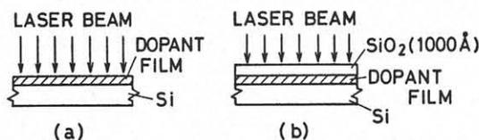
Fig. 1 Cross section of samples used for laser-doping.
