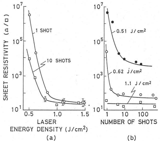
Fig. 4 (a) The dependence of sheet resistivity on laser energy density(a), and number of laser shots(b). SiO<sub>2</sub>(1000Å)/boron-coated Si was exposed to a stationary pulsed laser beam.
