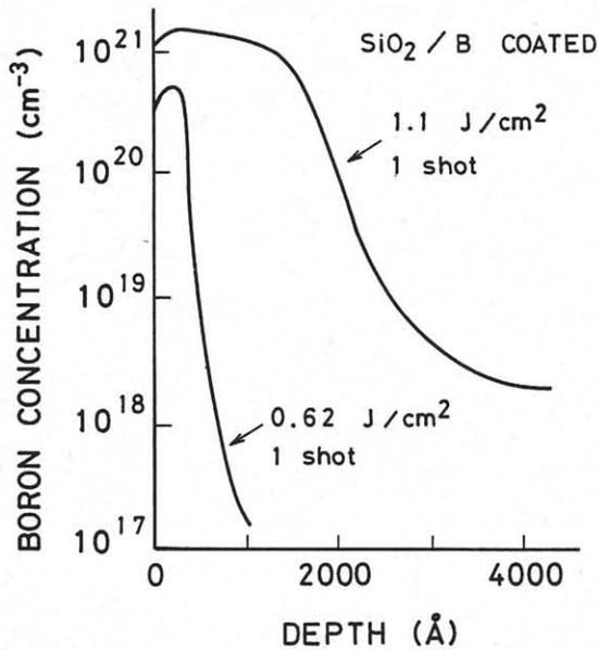
Fig. 5 Dopant profiles measured by SIMS.
