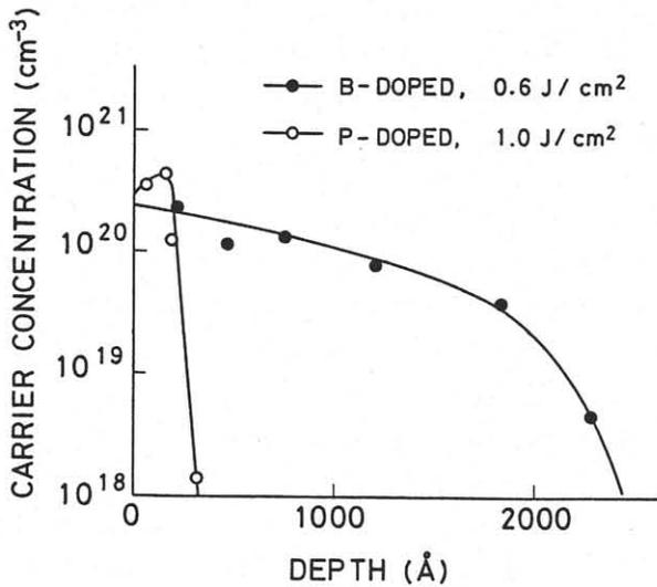
Fig. 3 Carrier concentration depth profiles for p<sup>+</sup>(solid circles) and n<sup>+</sup>(open circles) layers produced from boron/Si and phosphorus/Si samples, respectively.
