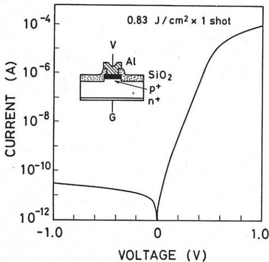
Fig. 6 I-V characteristics of a diode fabricated in the p<sup>+</sup> layer. The structure of the diode is shown in the inset.
