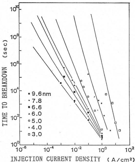
Fig. 1. Intrinsic breakdown lifetime vs. injection current density. Experimental and calculated results.
