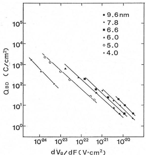
Fig. 2. Breakdown charge vs. trap generation rate
