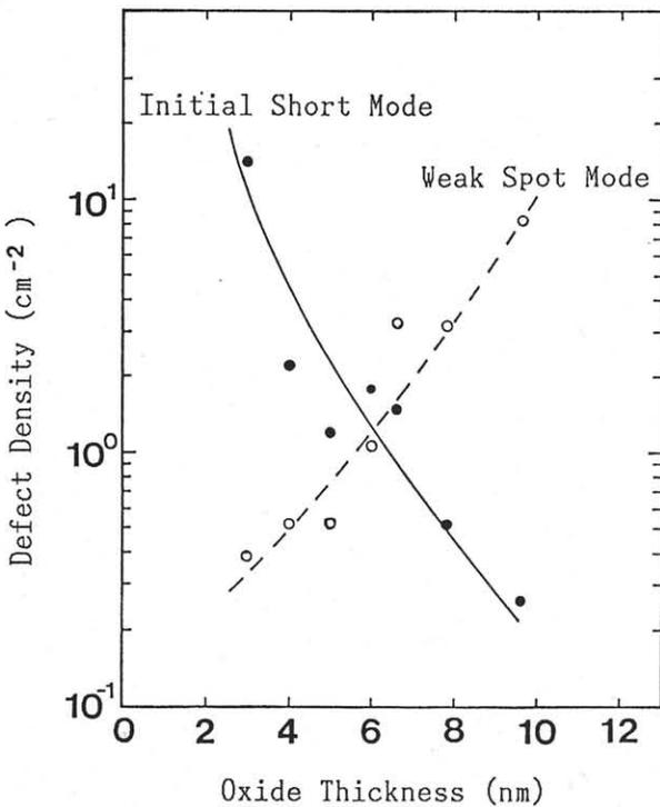
Fig. 3. Oxide defect density vs. oxide thickness.
