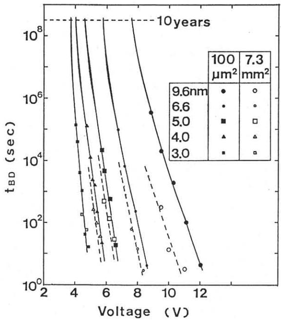
Fig. 4. The time to 50% failure (TDDB) of  $7.3 \text{ mm}^2$  capacitors and the intrinsic breakdown lifetime of  $100 \mu\text{m}^2$  capacitors vs. gate voltage.
