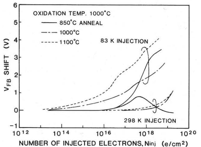
Fig.3 POA temperature dependence of flat-band voltage shifts due to electron injection
