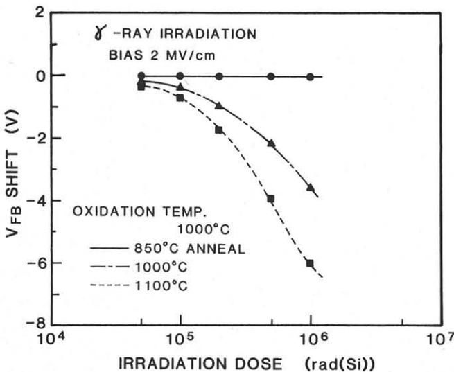
Fig.2 Flat-band voltage shifts due to gamma-ray irradiation under constant gate-bias of 2 MV/cm
