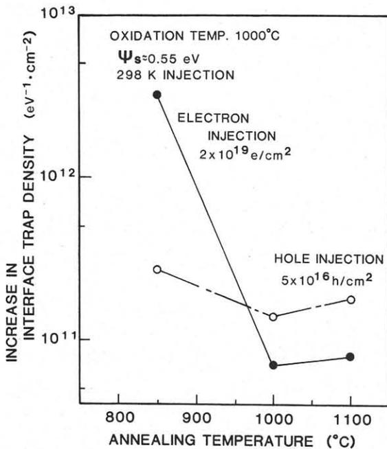
Fig.4 Increase in interface trap density due to hole and electron injection at 298 K
