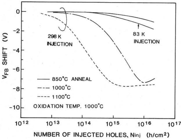
Fig.1 POA temperature dependence of flat-band voltage shifts due to hole injection
