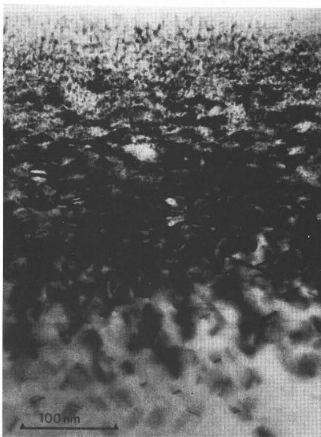
Fig.7. (110) cross-section of the silicon structure below the buried oxide
