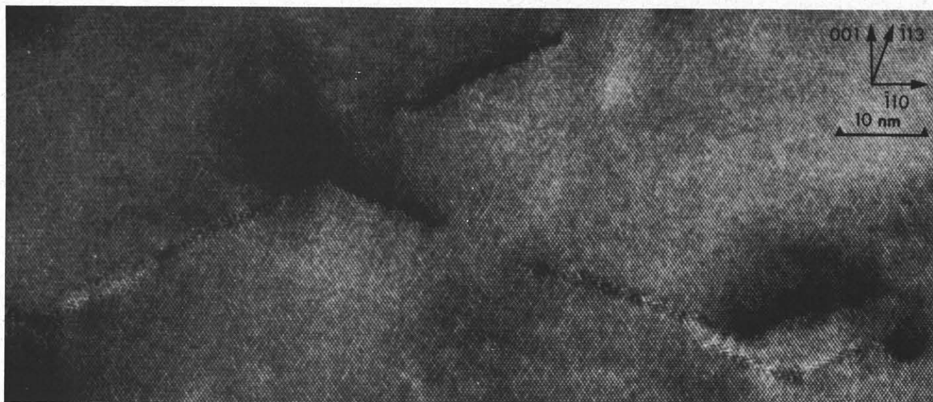
Fig.8. high resolution micrograph of plate-like coesite precipitates in silicon
