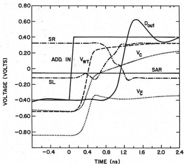
Fig. 5 Simulated internal waveforms of the 5-KBit RAM circuits.
