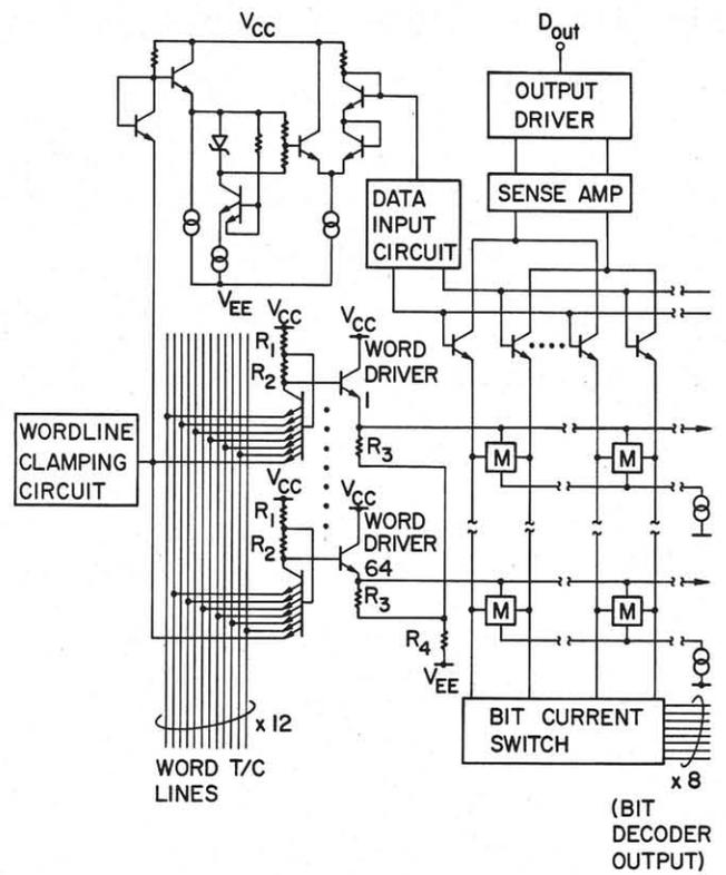
Fig. 3 Schematic diagram of the 5-KBit RAM.
