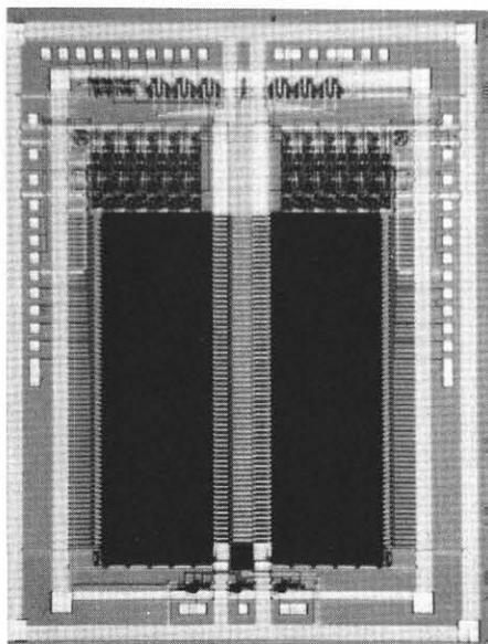
Fig. 6. Microphotograph of a 5-KBit RAM.
