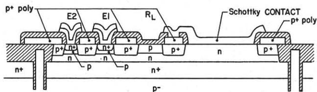
Fig. 2. Cross sectional view of the RAM cell.
