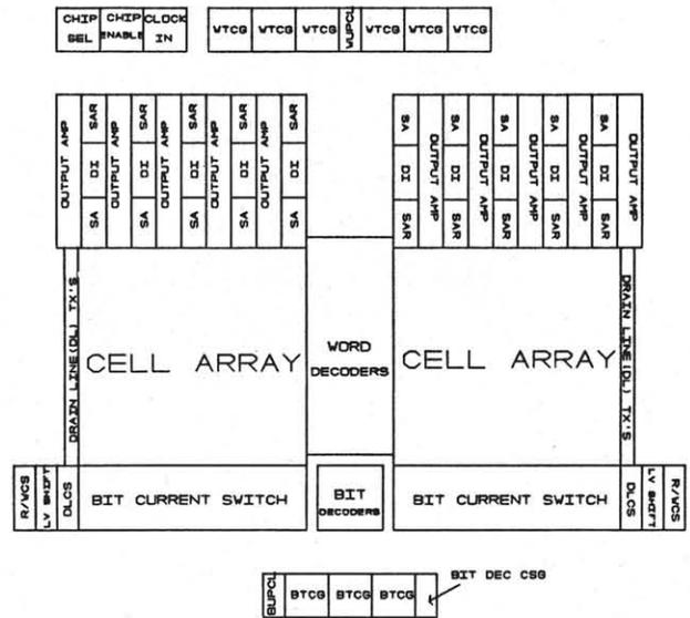
Fig. 4. Block diagram of the 5-KBit RAM.
