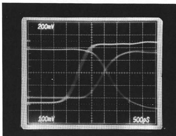
Fig. 7. Read access waveforms of the 5-KBit RAM.
