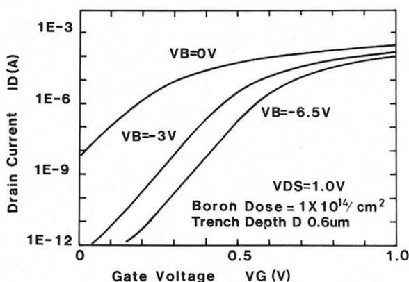
Fig.7 Sub-threshold characteristics of transfer gate transistor.
