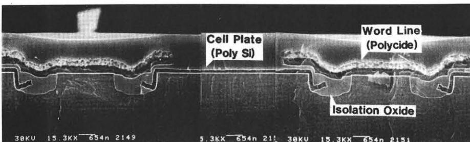
Fig.3 Cross sectional SEM photograph of PCC structure.
