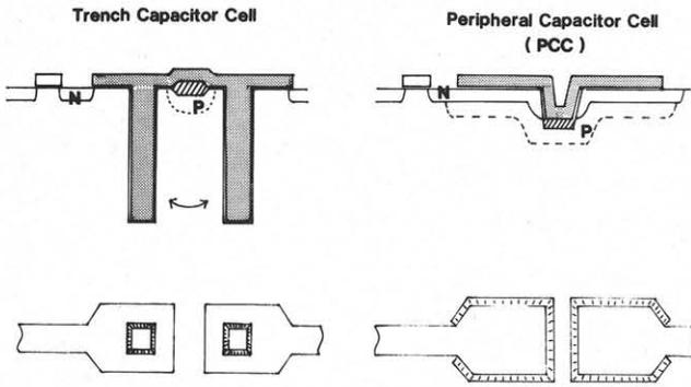
Fig.1 Schematic drawings of peripheral capacitor cell and trench capacitor cell
