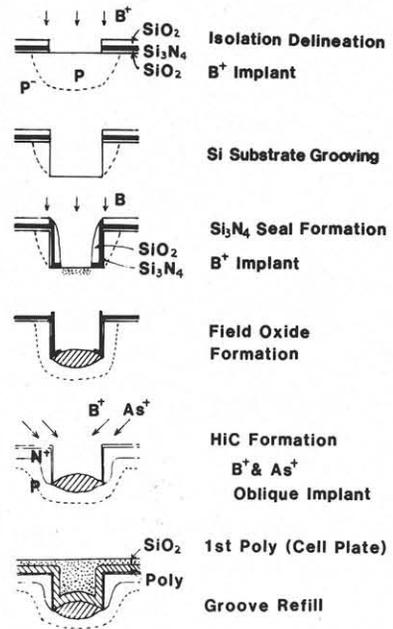
Fig.2 Fabrication process for PCC.
