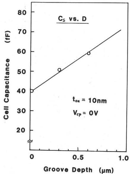
Fig.5 Storage capacitance vs. groove depth.
