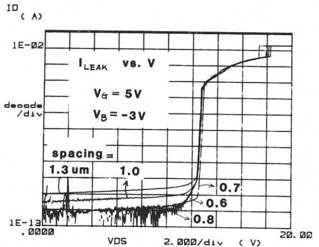
Fig.6 Cell to cell leakage current as a function of applied voltage.
