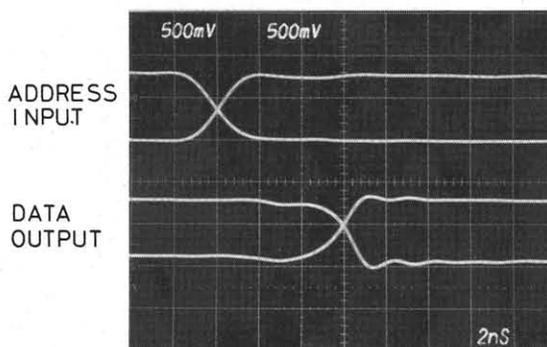
Fig. 7 Address access waveforms.
