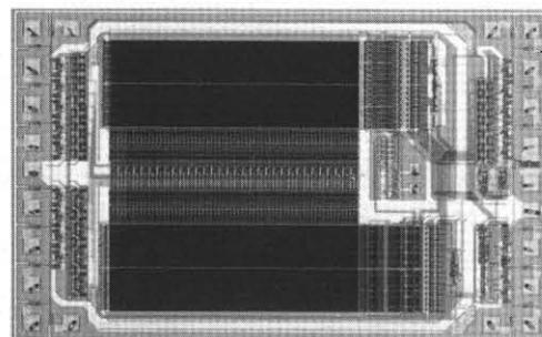
Fig. 6 Microphotograph of a 16Kb static RAM test chip.
