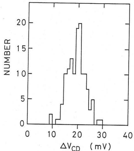
Fig. 5 Differential read voltage variations on the common data line.
