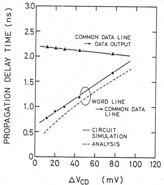
Fig. 4 Propagation delay time dependence on the common data line signal swing,  $\Delta V_{CD}$ .
