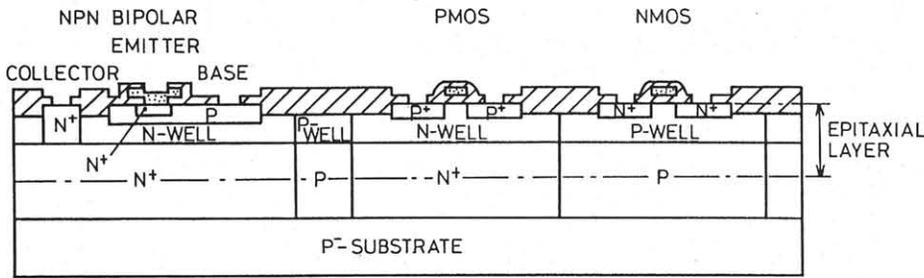
Fig. 1 Cross-section of the 1.3μm Hi-BiCMOS device.
