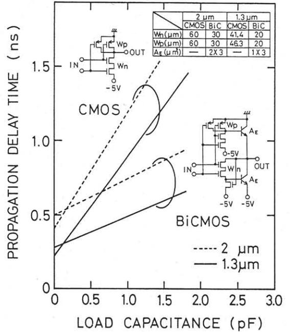
Fig. 2 Experimental propagation delay time of CMOS and BiCMOS 2 input NAND gates.
