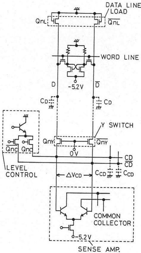
Fig. 3 Schematic diagram of memory cell and peripheral circuits of the data line and common data line.
