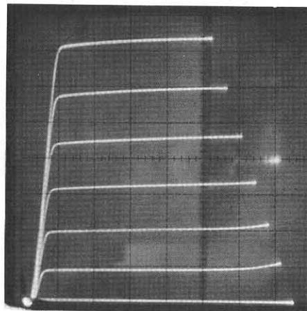
Fig.6:Emitter grounded I-V characteristics. I<sub>c</sub>:0.5mA/div., V<sub>c</sub>:1V/div., I<sub>b</sub>:20μA/div.
