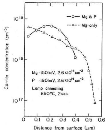
Fig.2: Depth profiles of carrier concentration for Mg-P and Mg-only implanted GaAs layers.
