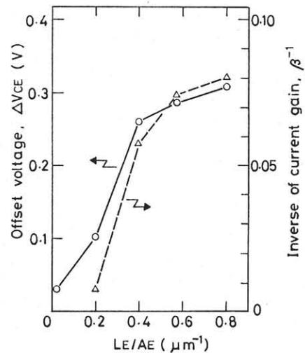
Fig.1: Collector-emitter offset voltage and inverse of current gain vs. emitter size. External base was formed by Mg-only implantation. Current gain was measured at  $10 \text{ kA/cm}^2$  collector current density.
