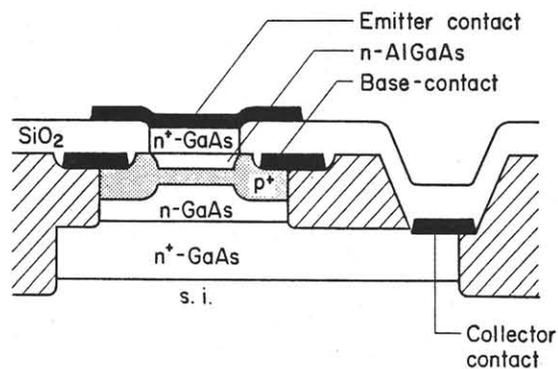
Fig.4:Self-aligned HBT cross-sectional view.
