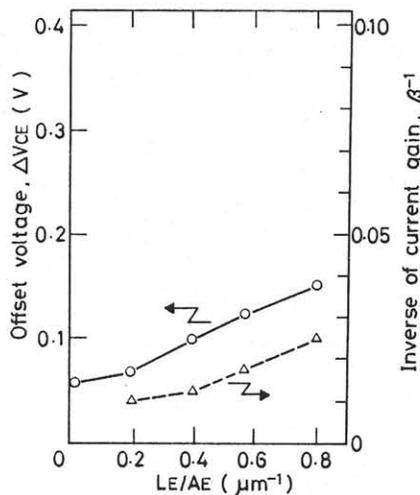
Fig.3:Collector-emitter offset voltage and inverse of current gain vs. emitter size. External base was formed by Mg and P double implantation. Current gain was measured at 10kA/cm<sup>2</sup> collector current density.
