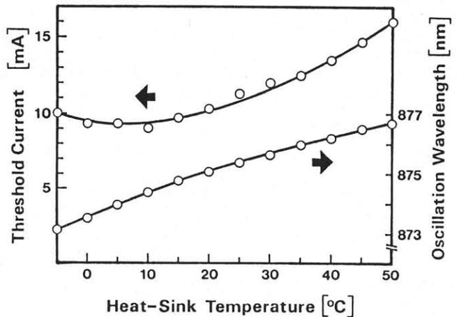
Fig.3. Dependence of the lasing wavelength and the threshold current on heat-sink temperature.
