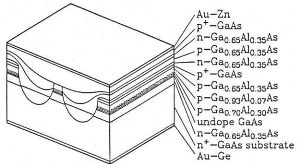
Fig.1. A schematic view of the GaAlAs/GaAs DFB DC-PBH LD.
