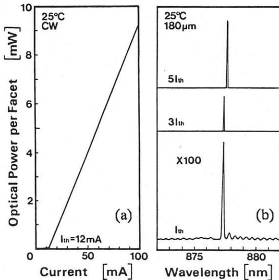
Fig.2. (a) Light output vs. injection current characteristics at room temperature, (b) Oscillation spectra at several injection levels
