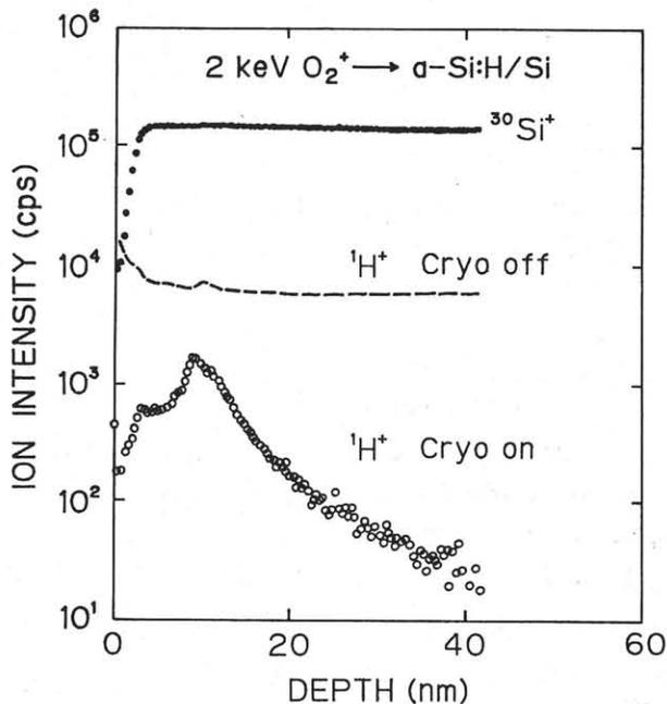
Fig. 3 Depth profile of H in 10 nm a-Si layer on Si measured by weak  $\text{O}_2^+$  beam.
