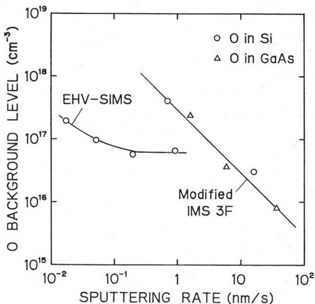
Fig. 4 Relationship between O background level and sputtering rate. Data obtained by the EHV-SIMS instrument are compared with those obtained by the cryopanel-equipped IMS-3F.
