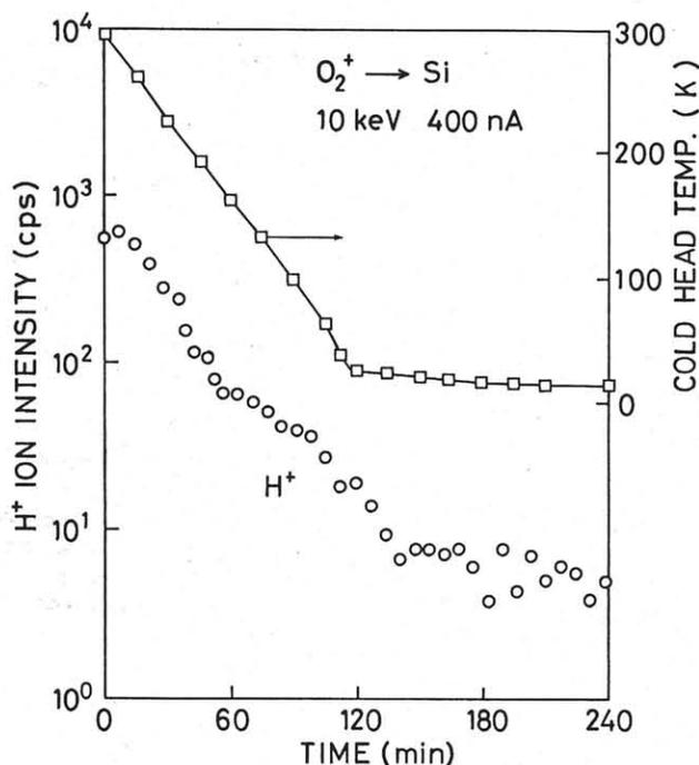
Fig. 1 Variation in H background signal under  $O_2^+$  bombardment after beginning of refrigeration process.
