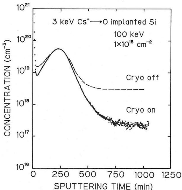
Fig. 2 Depth profiles of O-implanted in Si measured by weak  $\text{Cs}^+$  beam. The profile obtained during the cryopanel operation and that obtained without cryopanel operation are compared.
