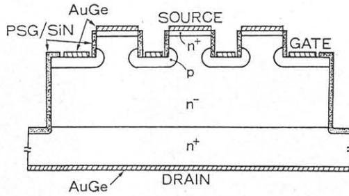
Fig. 1. Recessed gate SIT structure.
