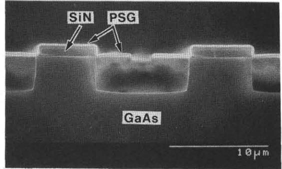
(b) Anisotropic etching of GaAs
