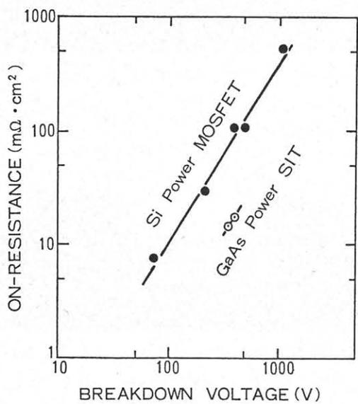
Fig. 5. On-resistance comparison between GaAs power SIT and Si power MOSFET.
