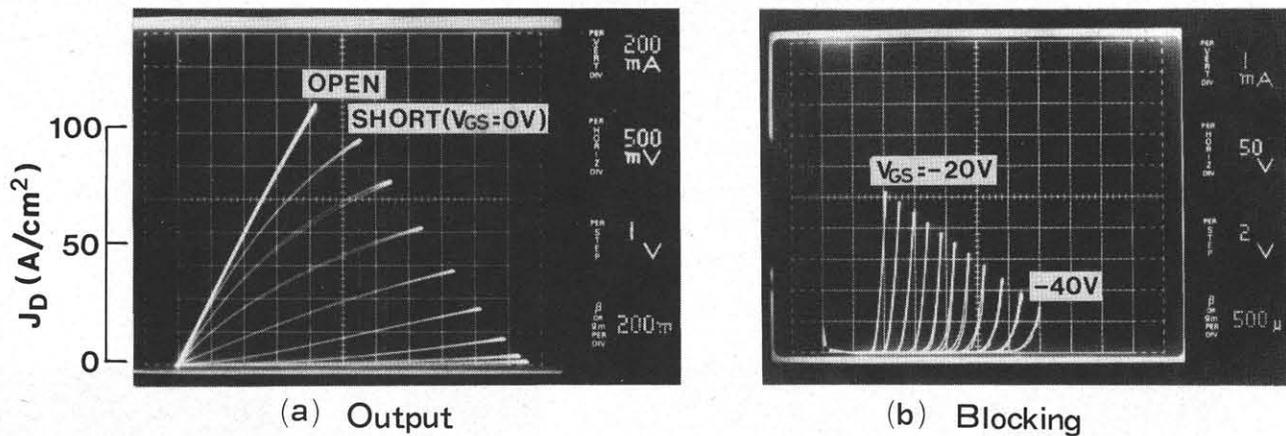
Fig. 4. I-V characteristics of GaAs power SIT.
