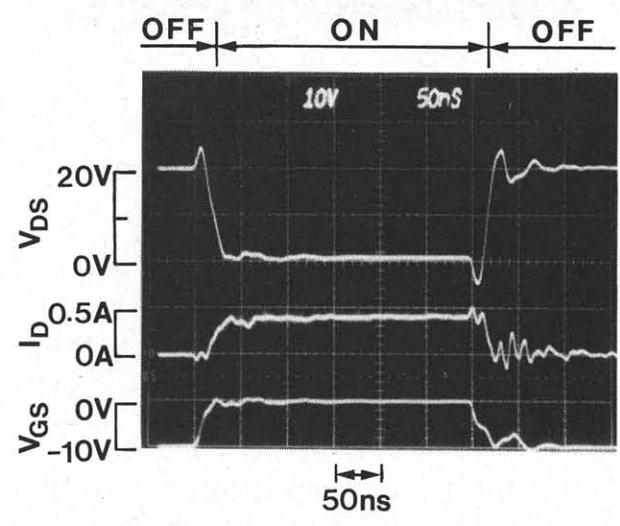
Fig. 6. Switching waveforms for GaAs power SIT.
