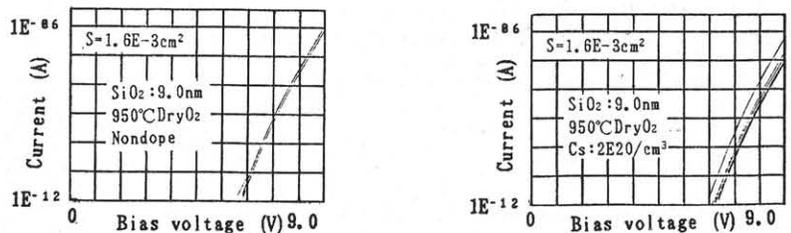
Fig. 4 I-V Characteristics of SiO<sub>2</sub>
