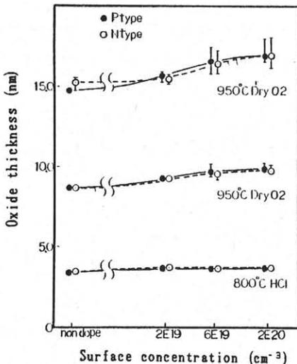
Fig. 3 Oxide thickness vs. Surface concentration
