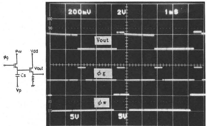
Fig. 9 Test circuit and waveforms for basic cell operation
