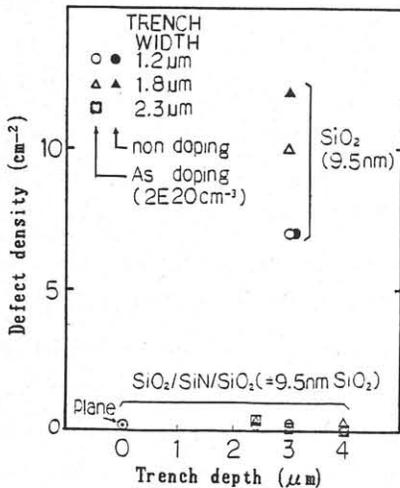
Fig. 6 Defect density of SiO<sub>2</sub>, SiO<sub>2</sub>/SiN/SiO<sub>2</sub> stacked dielectric film
