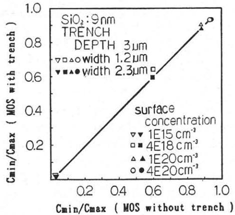
Fig.1 C<sub>min</sub>/C<sub>max</sub> of MOS with and without trench
