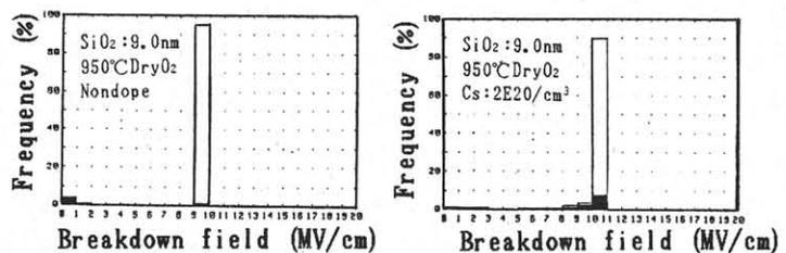
Fig. 5 Oxide breakdown voltage histograms
