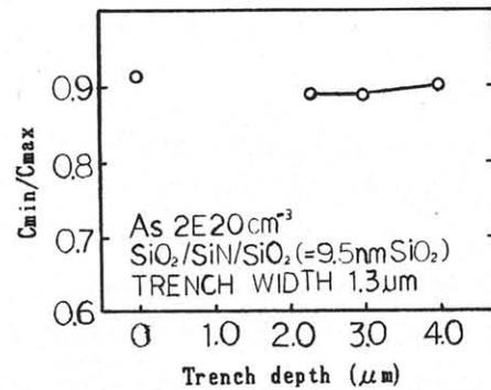
Fig.2 Dependence of C<sub>min</sub>/C<sub>max</sub> on trench depth
