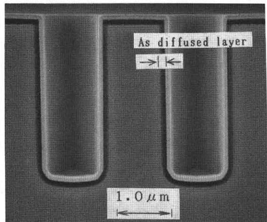
Photo 1 Cross sectional view of SEM on As diffused layer in trench
