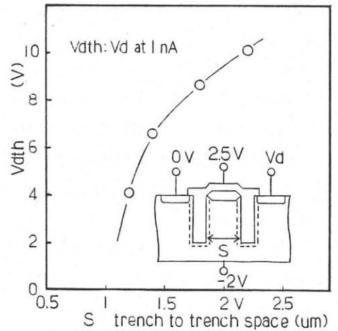
Fig. 8 Voltage at 1nA trench to trench leakage current
