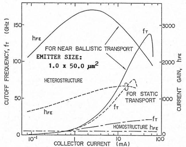
Fig. 6  $f_T$  and  $h_{FE}$  versus collector current in HBTs.
