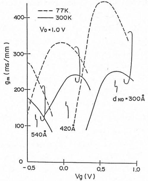
Fig. 5 Dependence of  $g_m$  on gate lengths in HEMTs.
