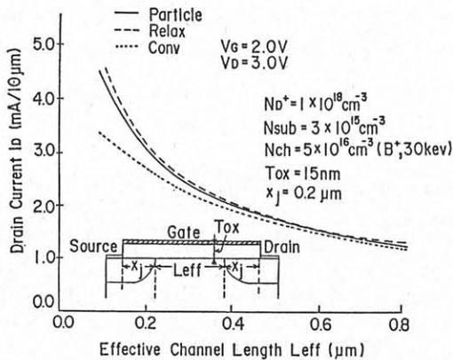
Fig. 3 Drain current versus effective channel length for three different approaches in Si MOSFETs.
