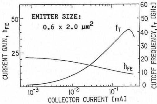
Fig. 2  $f_T$  and  $h_{FE}$  characteristics versus collector current in Si npn transistor.
