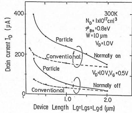
Fig. 4 Drain currents versus device length in GaAs MESFETs.
