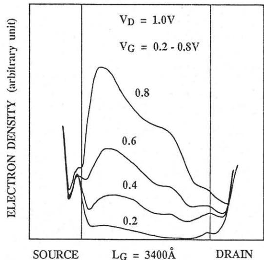
Fig.2 The density profiles of 2DEG plus electrons which situate in the  $\Gamma$ -valley and within  $200\text{\AA}$  from the heterointerface.  $V_d = 1.0\text{V}$ .  $V_g$  is varied from  $0.2\text{V}$  to  $0.8\text{V}$ .
