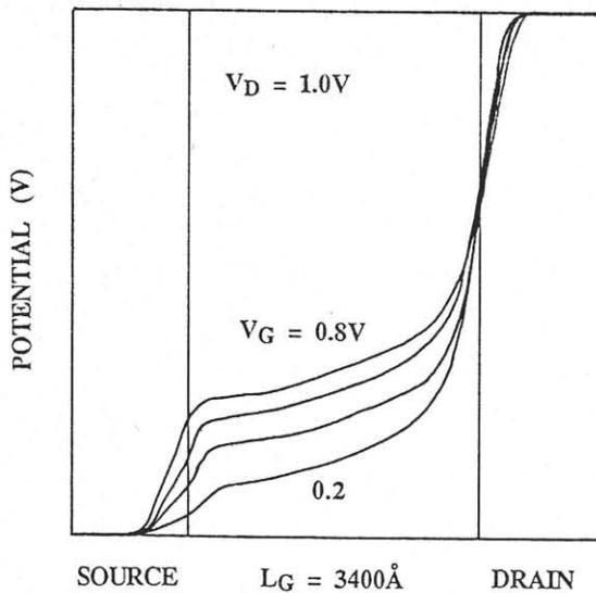
Fig.4 The potential profiles along the channel.  $V_g$  is varied from  $0.2\text{V}$  to  $0.8\text{V}$ .  $V_d = 1.0\text{V}$ .
