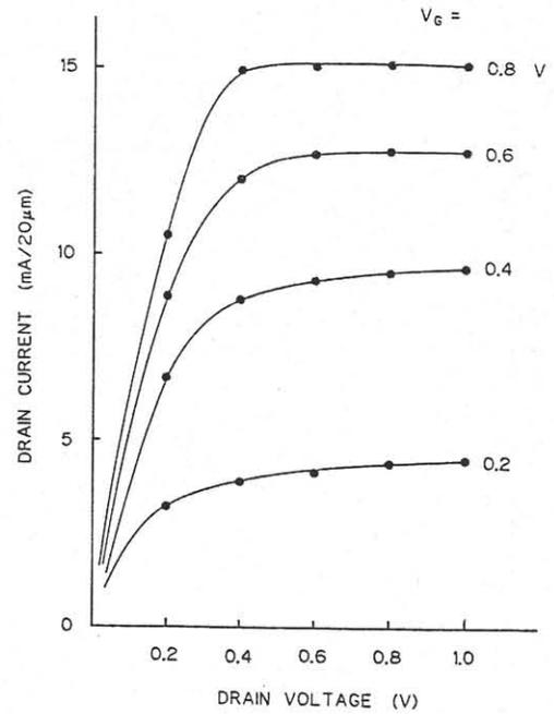
Fig.5 The current-voltage characteristics of  $0.34\mu\text{m}$ -long gate FET.  $D=175\text{\AA}$ .
