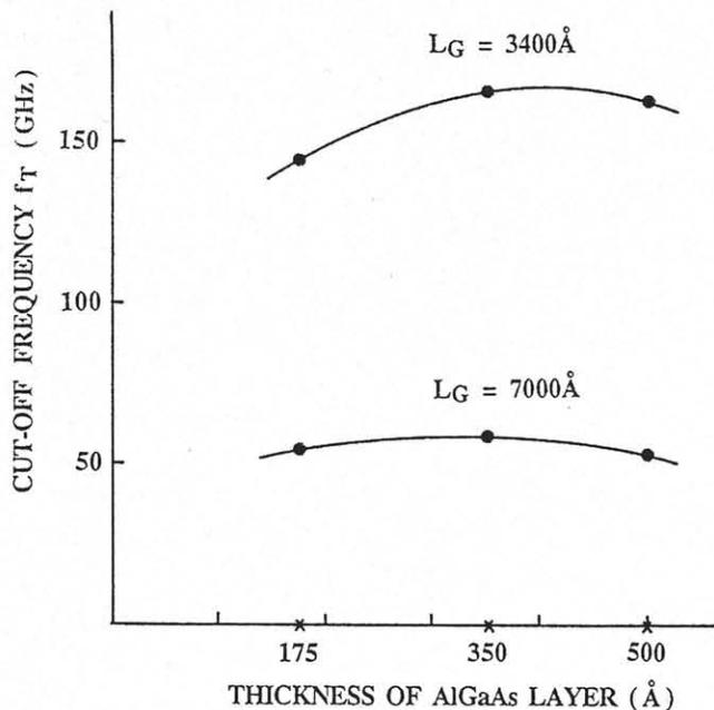
Fig.6 The unity-current-gain cut-off frequency of MIS-like FETs.
