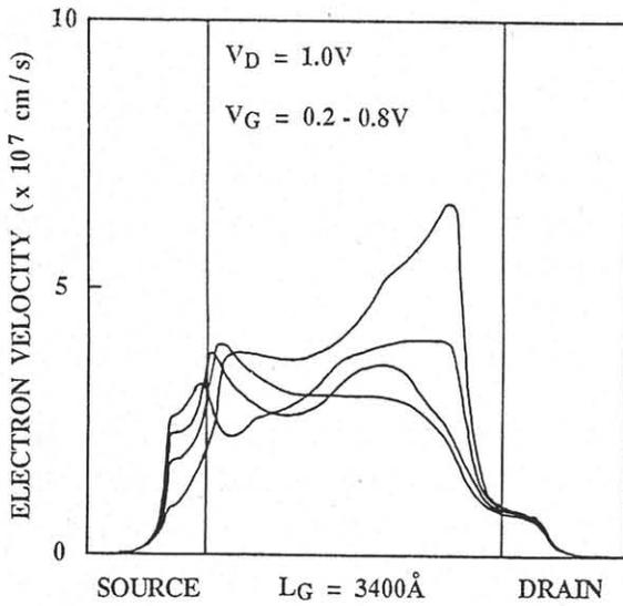
Fig.3 The profiles of the mean velocity of 2DEG plus electrons which situate in the  $\Gamma$ -valley and within  $200\text{\AA}$  from the heterointerface in the channel.  $V_g$  is varied from  $0.2\text{V}$  to  $0.8\text{V}$ .  $V_d = 1.0\text{V}$ .
