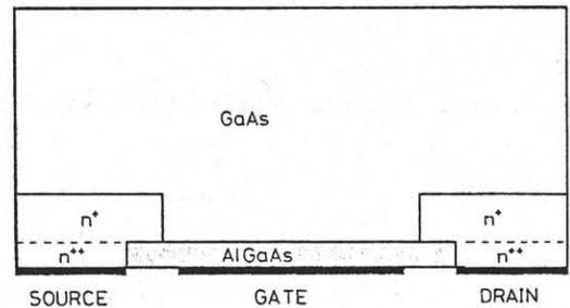
Fig.1 Model of heterostructure MIS-like FET. The doping densities of  $n^+$  and  $n^{++}$  layers are  $5 \times 10^{17} \text{ cm}^{-3}$  and  $1 \times 10^{18} \text{ cm}^{-3}$ , respectively. The gate length  $L_g$  is either  $0.34\mu\text{m}$  or  $0.7\mu\text{m}$ . The thickness of AlGaAs semi-insulating layer  $D$  is varied from  $175\text{\AA}$  to  $500\text{\AA}$ . The lattice temperature  $T$  is assumed to be  $77\text{K}$ .
