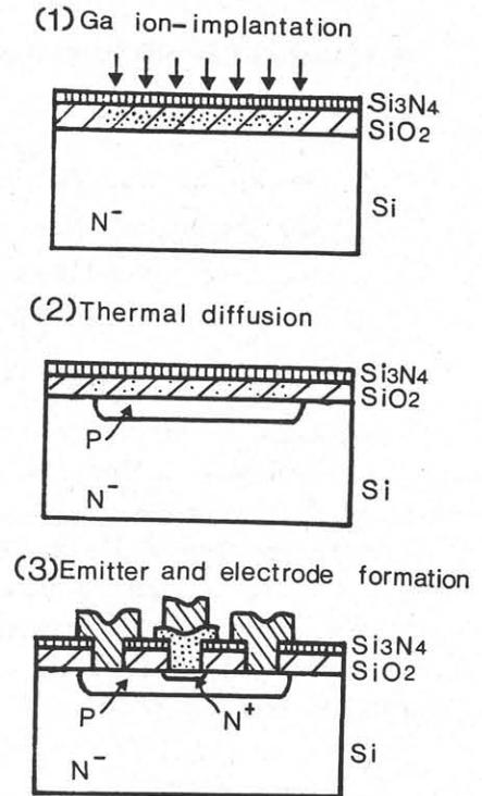
Fig.2 Fabrication steps of gallium base transistor.
