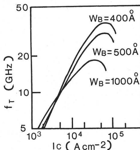
Fig.1 Performance expectation of a Si bipolar transistor.
