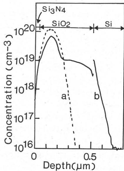
Fig.3 Typical example of gallium diffusion in the Si<sub>3</sub>N<sub>4</sub>/SiO<sub>2</sub>/Si structure.
