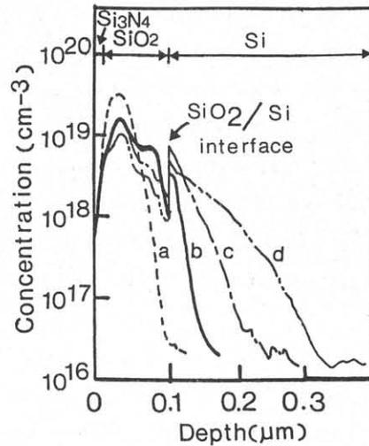
Fig.4 Gallium profiles at 900°C by a:0min, b:20min, c:60min, d:240min heat treatment.
