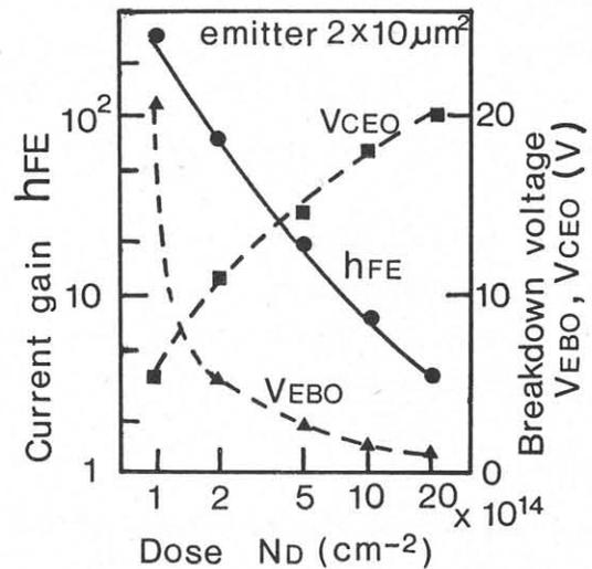
Fig.5 Transistor parameters ( $h_{FE}$  and breakdown voltages) for various gallium dose.
