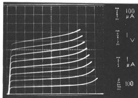
Fig.6 Typical  $I_C$ - $V_{CE}$  characteristics ( $V:100\mu\text{A}/\text{div}, H:1\text{V}/\text{div}, 1\mu\text{A}/\text{step}$ )
