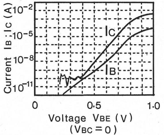
Fig.7 Typical Gummel plot of the transistor.
