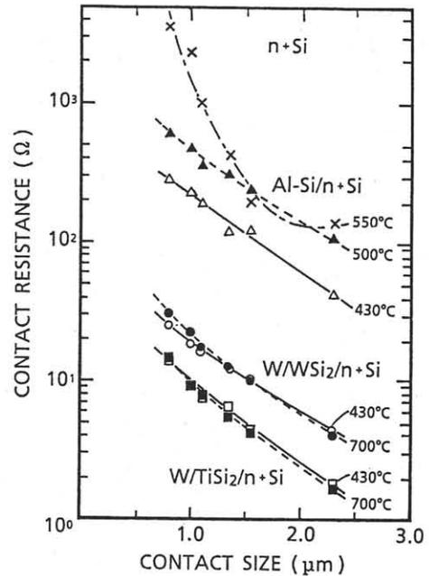
Fig.5 Contact resistance as a function of contact size, comparing after 430°C and higher temperature annealing.
