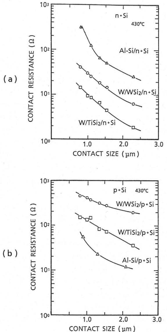
Fig.2 Contact resistance after 430°C annealing, as a function of contact size, (a) n<sup>+</sup>Si, (b) p<sup>+</sup>Si.
