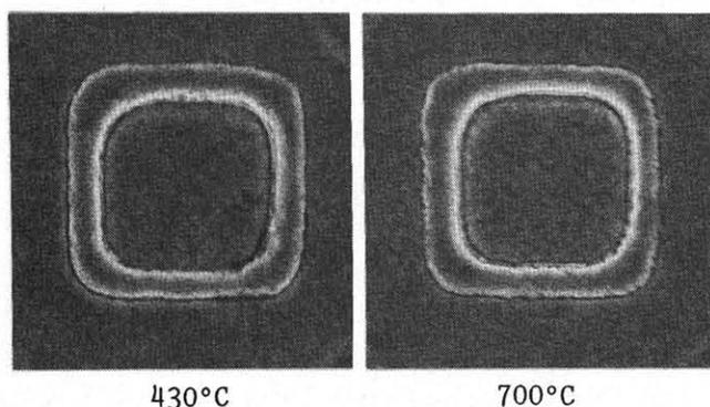
Fig.7 SEM micrographs of W/TiSi<sub>2</sub>/Si contact surface, after 430°C and 700°C annealing.
