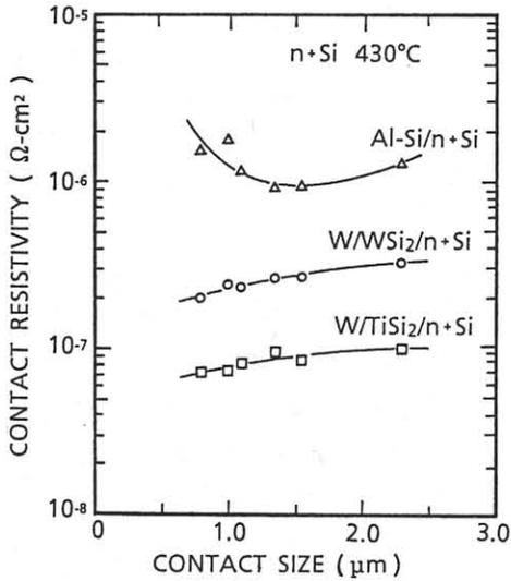
Fig.3 Contact resistivity after 430°C annealing, as a function of contact size.
