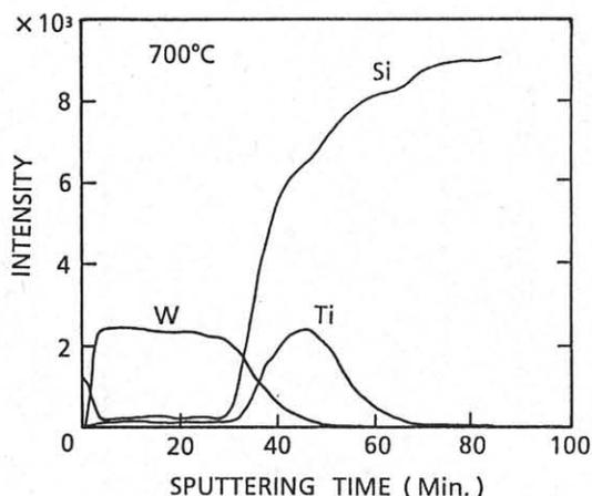
Fig.6 AES depth profile of W, Ti and Si in the W/TiSi<sub>2</sub>/Si structure after 700°C annealing.
