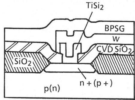
Fig.1 Cross section of W/TiSi<sub>2</sub>/Si contact structure.
