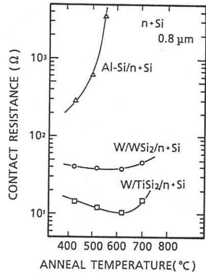
Fig.4 Contact resistance as a function of anneal temperature.
